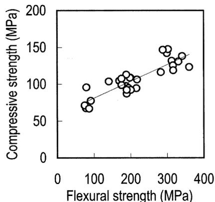
Fig. 4 Correlation of flexural strength and compressive strength.
