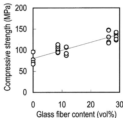
Fig. 3 Correlation of compressive strength and woven glass fiber content.
