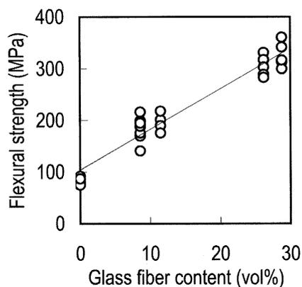
Fig. 2 Correlation of flexural strength and woven glass fiber content.
