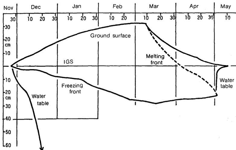
Fig. 1 Frost penetration sequence as functions of time and depth measured from the initial ground surface (IGS), showing ground surface heave, melting front, freezing front and water table. From November 1976 to May 1977, at Tomakomai field site.
