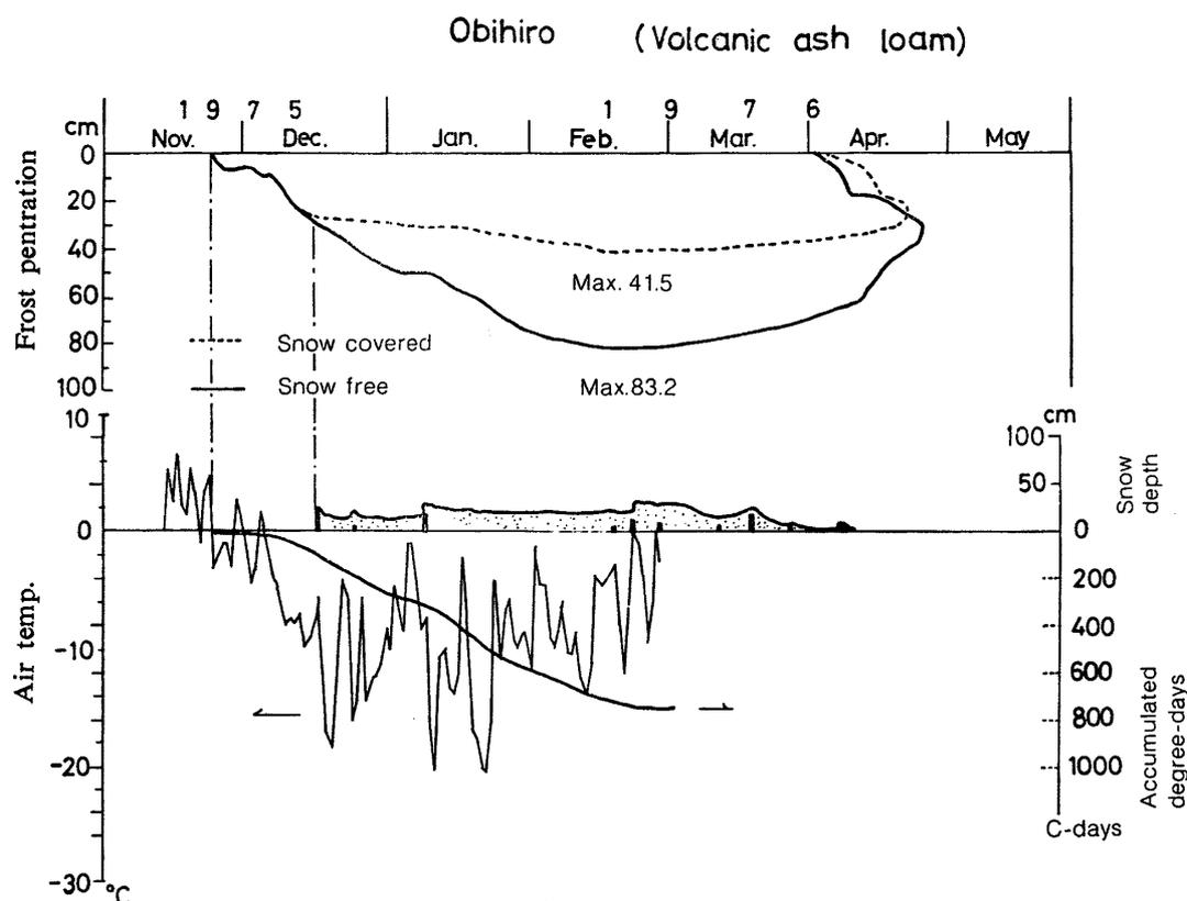
Fig. 4 Frost penetration sequence as function of time at campus of Obihiro University, showing snow covered and snow free cases, plus snow depth, daly mean air temperature and accumulated degree-days.
