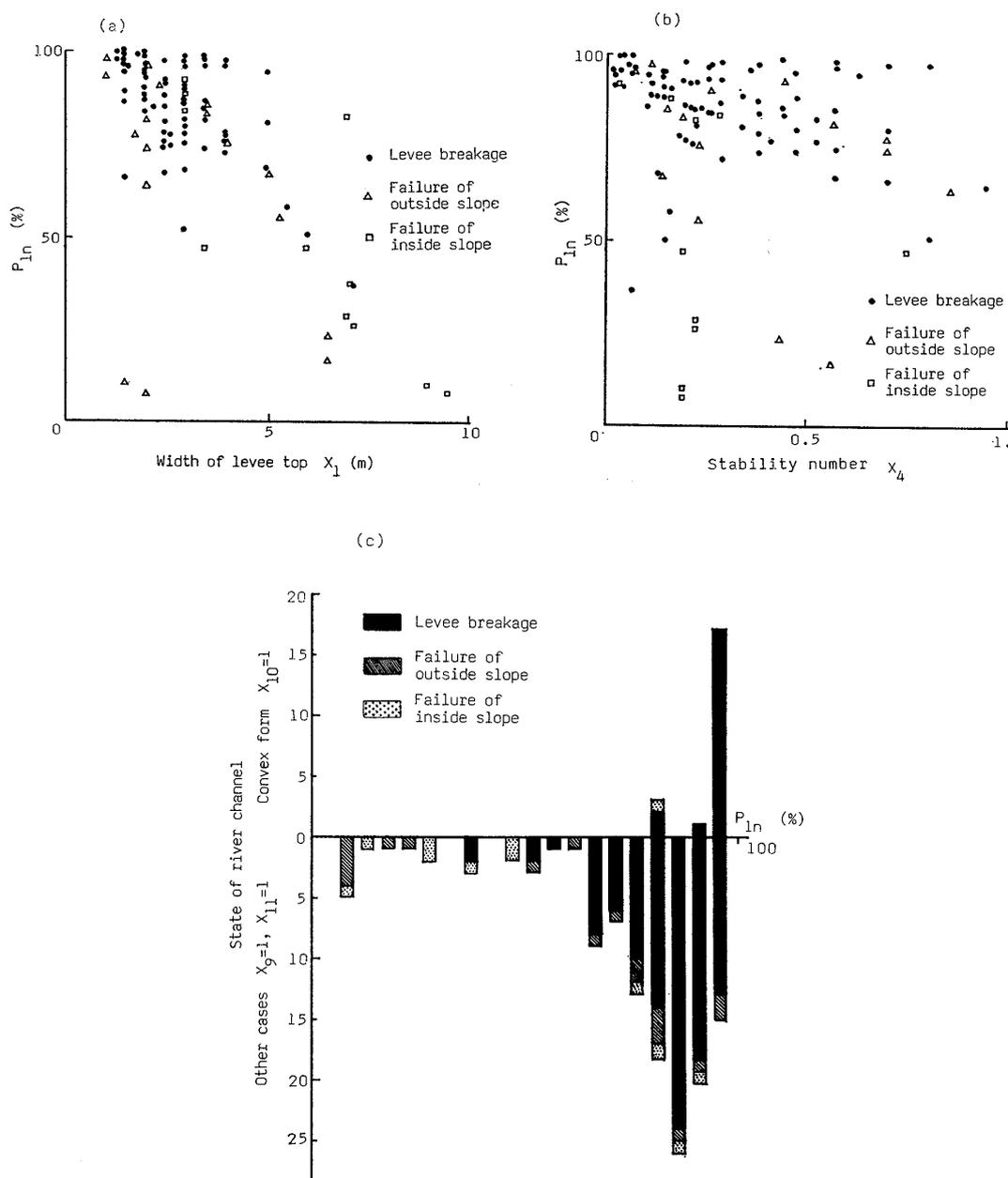
Fig. 8 Effect of factors on the probability of collapse; model 2. (a) Width of the levee top ( $X_1$ ); (b) Soil strength parameter, stability number ( $X_4$ ); and (c) State of the river channel, convex form ( $X_{10}$ ).
