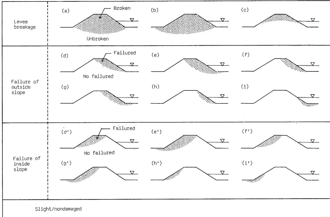
Fig. 1 Four types of levee collapse.
