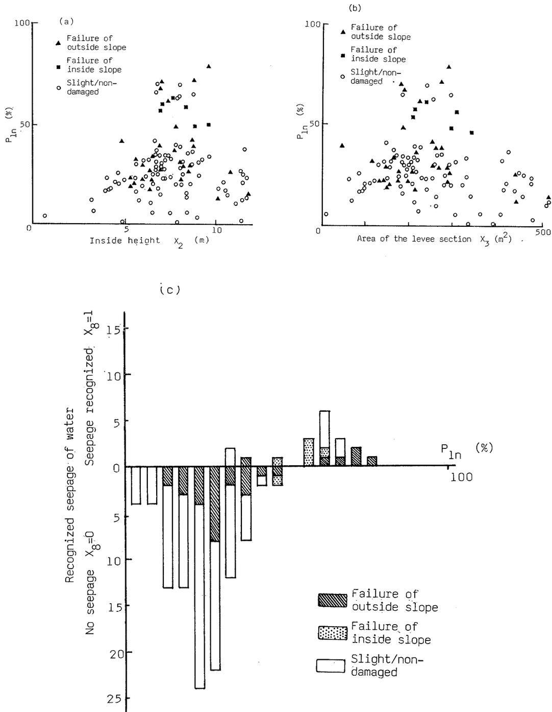
Fig. 10 Effect of factors on the probability of collapse; model 4. (a) Inside height ( $X_2$ ), (b) Area of the levee section ( $X_3$ ), and (c) Recognized seepage water ( $X_8$ ).
