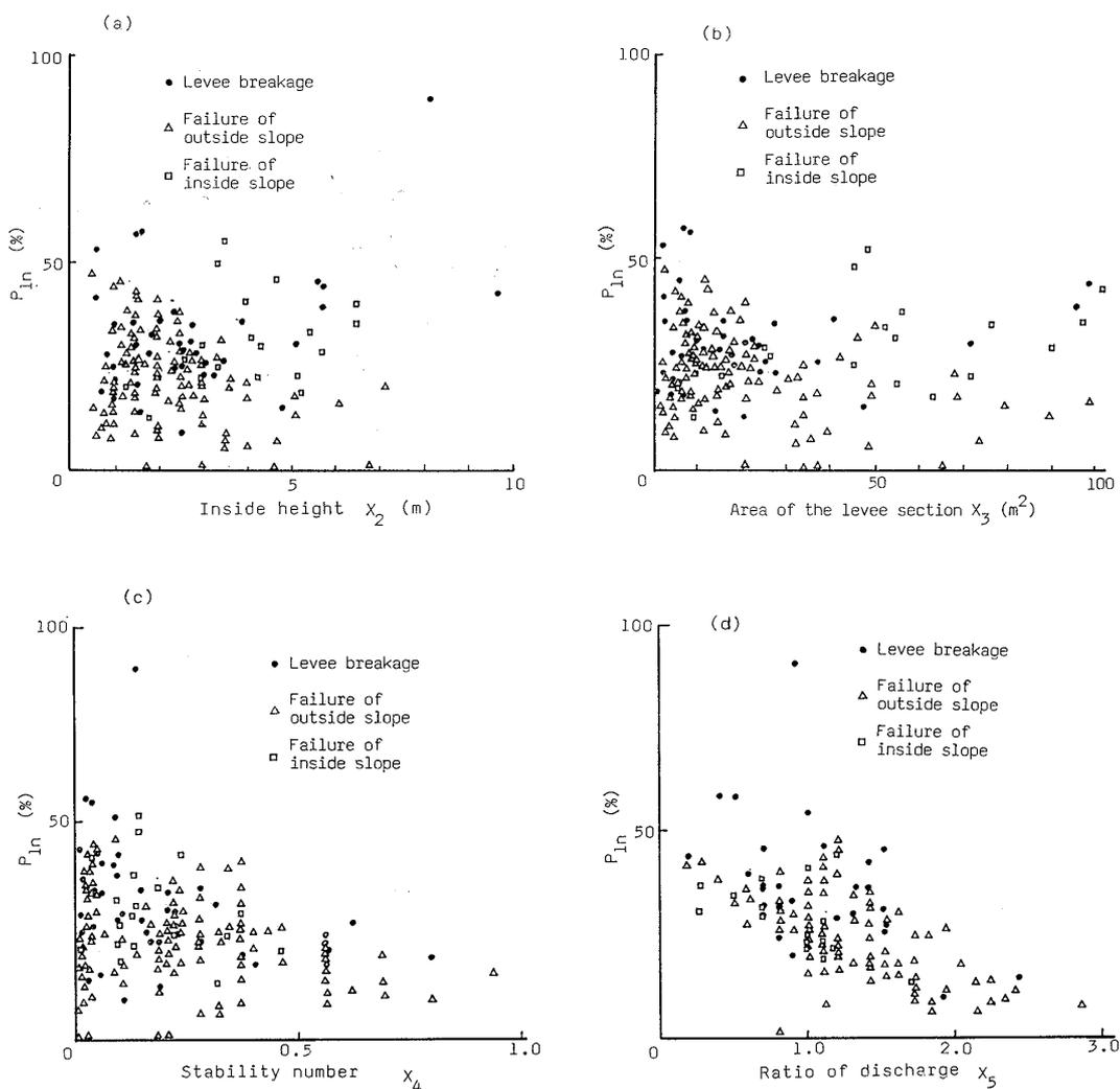
Fig. 9 Effect of factors on the probability of collapse; model 3. (a) Inside height ( $X_2$ ), (b) Area of the levee section ( $X_3$ ), (c) Stability number ( $X_4$ ), and (d) Ratio of discharge ( $X_5$ ).
