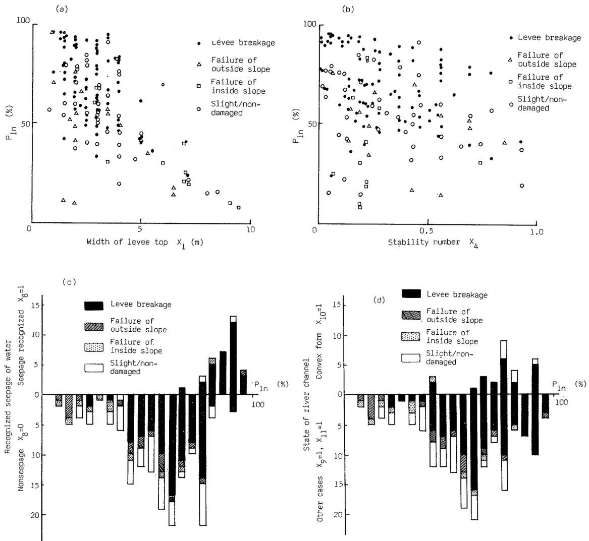
Fig. 2 Effect of factors on the probability of collapse; model 1. (a) Width of the levee top ( $X_1$ ), (b) Soil strength parameter; stability number ( $X_4$ ), (c) Recognized seepage water ( $X_8$ ), and (d) State of the river channel; convex form ( $X_{10}$ ).
