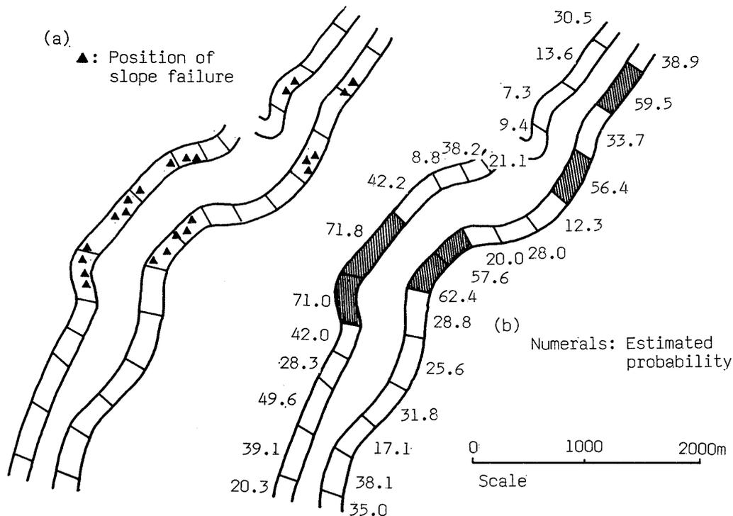
Fig. 11 Correspondence of actual positions of slope failure to sectional positions that had more than a 50% estimated probability of collapse.
