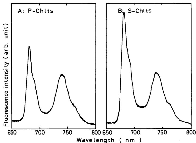
**Fig. 2** Low temperature (77 K) fluorescence emission spectra of P-Chlts (A) S-Chlts (B). Chloroplasts were suspended in 0.4 M sucrose, 10 mM NaCl, 5 mM MgCl<sub>2</sub> and 20 mM HEPES-KOH (pH 7.0). Chl *a/b* ratio of P- and S-Chlts were 3.41 and 2.75, respectively.
