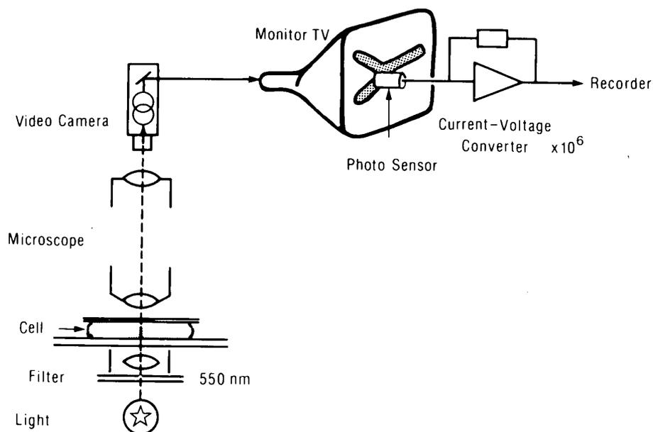
**Fig. 1** Schematic diagram of the system for recording chloroplast translocation. For details, see text.
