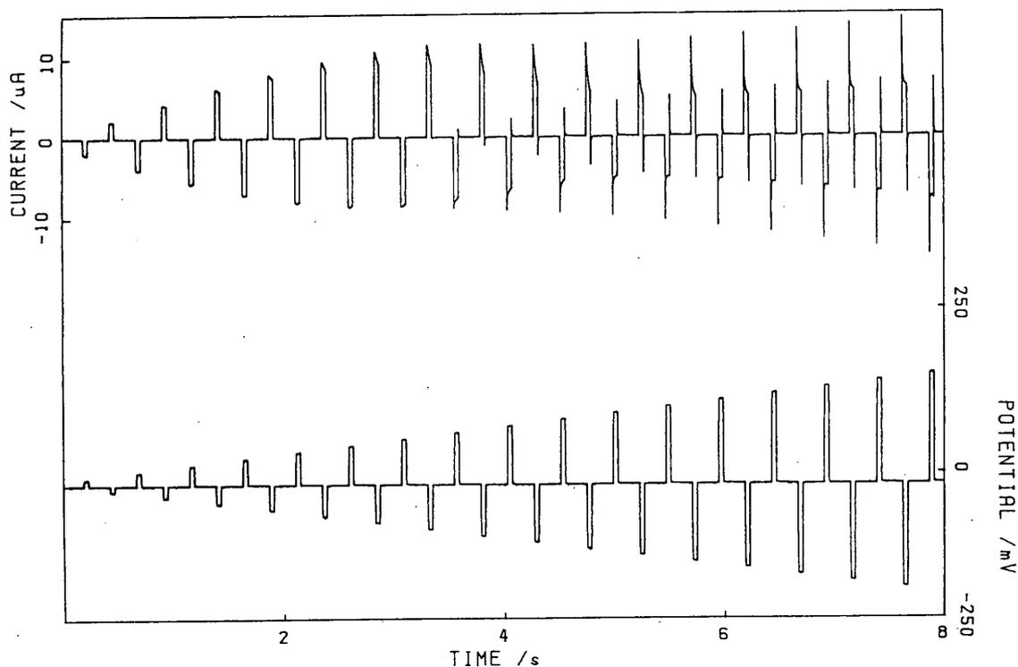
**Fig. 2** A typical bipolar staircase of voltage clamp commands (lower trace), with resulting current (upper trace). The cell is in ice cold high  $Cl^-$  permeabilising solution without ATP or  $PP_i$ ; cell surface area  $18 \text{ mm}^2$ . Note the inductive behaviour at low potential displacements, and capacitive later on.
