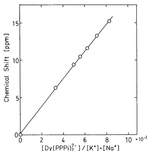
**Fig. 1** Effect of  $\text{Dy}(\text{PPPi})_2^{7-}$  on  $^{39}\text{K}$  NMR chemical shift of the  $\text{K}^+$  resonance. The chemical shift of  $\text{K}^+$  resonance shifted to higher magnetic field was measured relative to the chemical shift of the KCl solution as an external reference (0 ppm).
