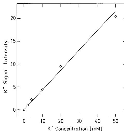
**Fig. 3** Relationship between  $\text{K}^+$  concentration and integrated  $\text{K}^+$  signal intensity in  $^{39}\text{K}$  NMR spectra. The  $\text{K}^+$  signal intensity represents relative intensity of  $\text{K}^+$  resonance in the standard KCl solution.
