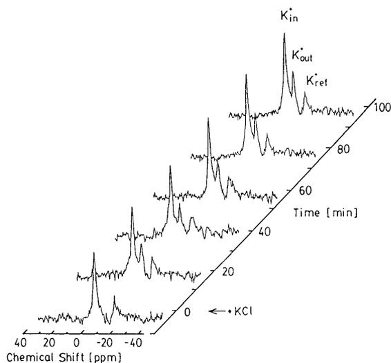
**Fig. 5** Changes of  $^{39}K$  NMR spectra by addition of 20 mM KCl. The root tips were firstly perfused with the solution containing  $2.5 \text{ mM Dy}(\text{PPP}_i)_2^-$ . Then 20 mM KCl was added to external solution at time 0 min.
