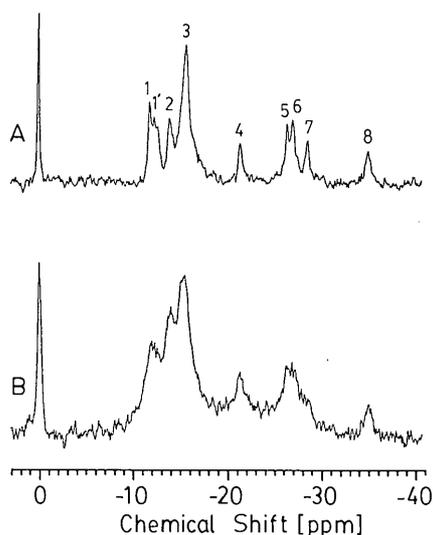
**Fig. 2** Effect of  $\text{Dy}(\text{PPP}_i)_2^{7-}$  on  $^{31}\text{P}$  NMR spectra of mung bean root tips. A: The spectrum before addition of  $\text{Dy}(\text{PPP}_i)_2^{7-}$ . B: The spectrum in 30 min after addition of 2.5 mM  $\text{Dy}(\text{PPP}_i)_2^{7-}$ . Peak assignments: 1, G6P; 2, cytoplasmic P<sub>i</sub>; 3, vacuolar P<sub>i</sub>; 4,  $\gamma$ -ATP; 5,  $\alpha$ -ATP; 6, UDPG and nicotinamide adenine nucleotides; 7, UDPG; 8,  $\beta$ -ATP. Peak 1' seemed to be F6P.
