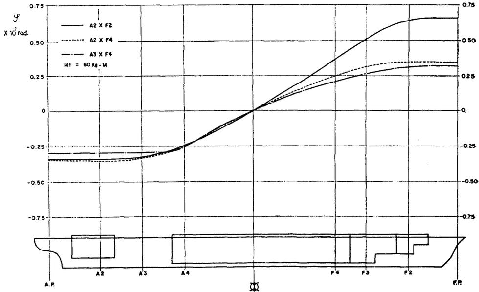
Fig. 25 Angle of Twist
