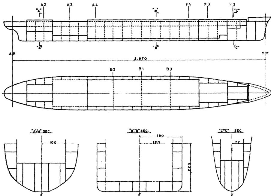
Fig. 22 Structure Plans of Model Ship
