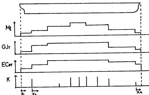
Fig. 30 Distributions of  $M_t$ ,  $GJ_T$ ,  $EC_{BT}$  &  $K$  for Ship's Hull Structure
