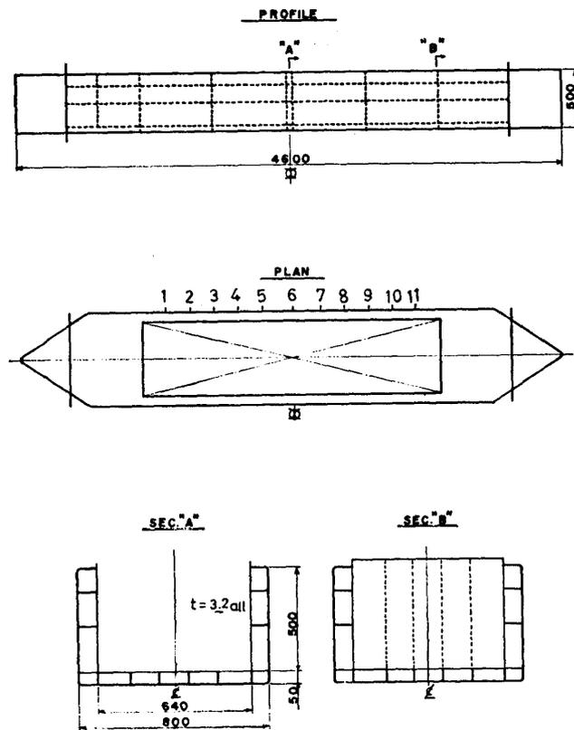
Fig. 6 Box Beam Model
