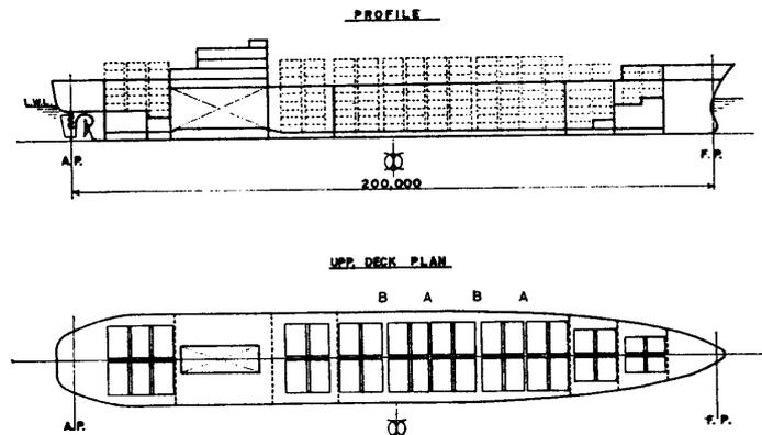
Fig. 32 a General Arrangement of Container Ship
