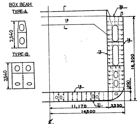
Fig. 32 b Midship Section of Container Ship
