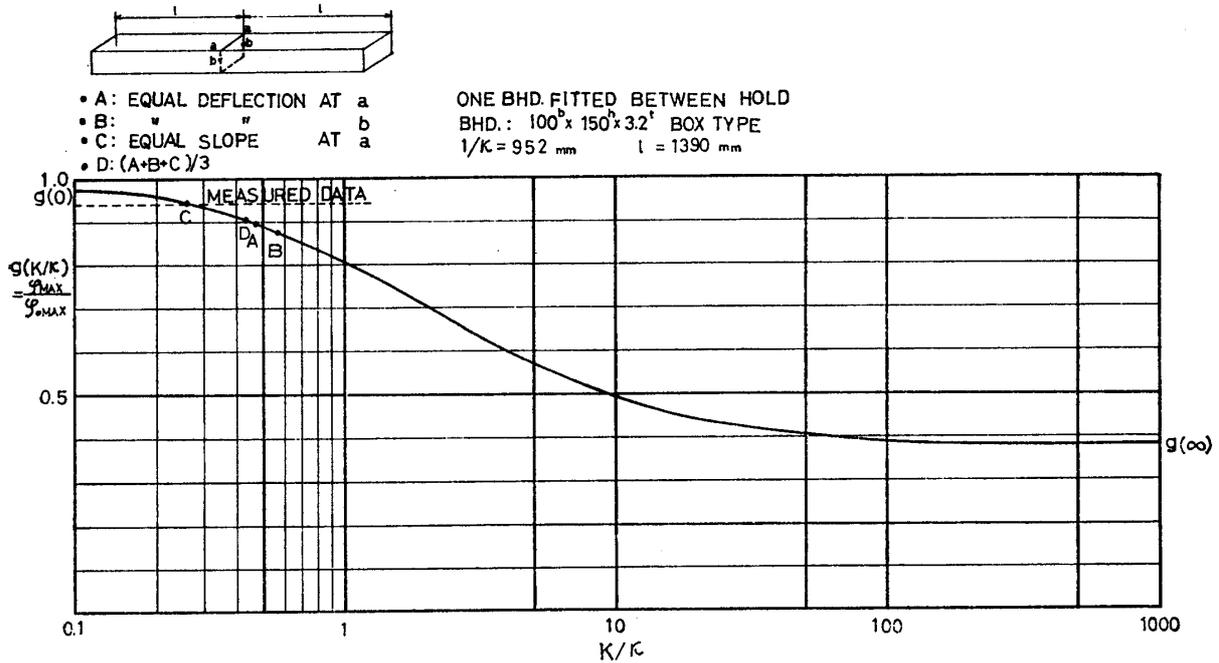
Fig. 21 Comparison of Theory and Experiment in Case of Box Beam Experiment
