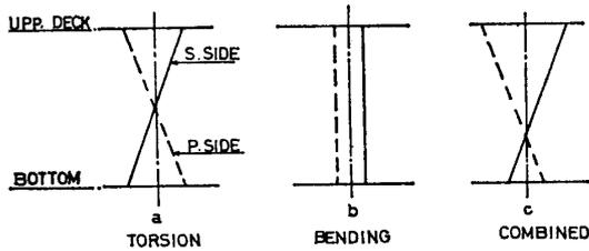
Fig. 13 Behaviour of BHD Displacement
