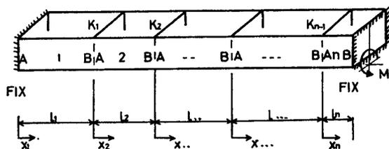
Fig. 20 Uniform Beam with U Shaped Section Having multiple Numbers of Elastic BHD.
