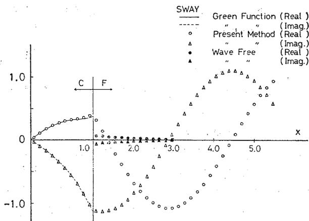
Fig. 3 Distribution of 1st-order potential on body and free-surface in swaying oscillation (circular cylinder,  $Kb=1.0$ )
