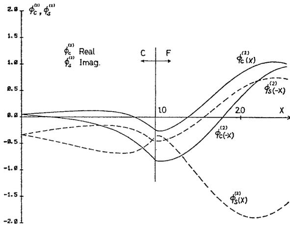
Fig. 5 Distribution of 2nd-order diffraction potential on body and free-surface (circular cylinder,  $Kb=0.5$ )
