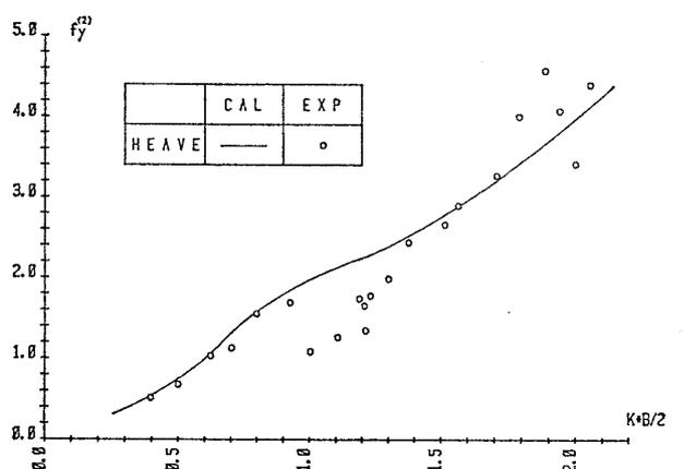
Fig. 12 2nd-order vertical wave exciting force (rectangular cylinder)
