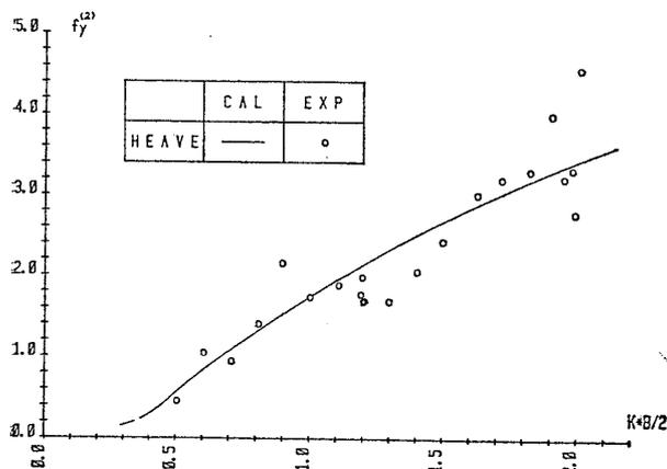
Fig. 10 2nd-order vertical wave exciting force (circular cylinder)
