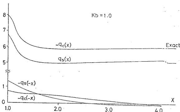
Fig. 4 Pressure distribution on free-surface in diffraction problem for circular cylinder ( $Kb=1.0$ )
