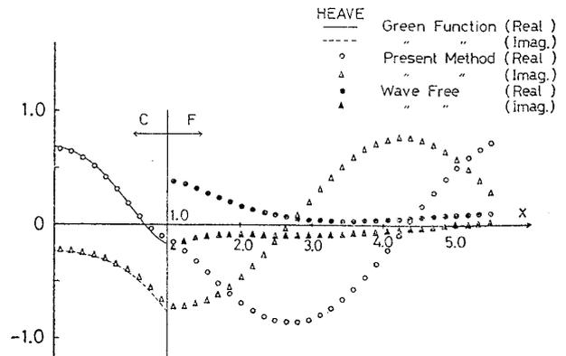
Fig. 2 Distribution of 1st-order potential on body and free-surface in heaving oscillation (circular cylinder,  $Kb=1.0$ )
