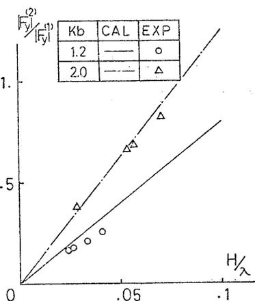
Fig. 14 Ratio of 2nd-order vertical force to that of 1st-order for various incident wave height (circular cylinder)
