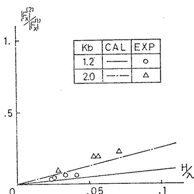
Fig. 15 Ratio of 2nd-order horizontal force to that of 1st-order for various incident wave height (circular cylinder)
