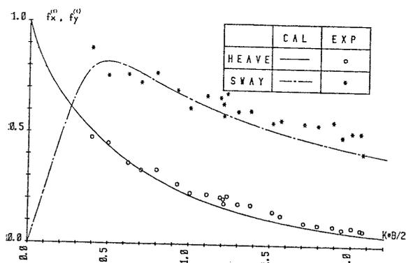
Fig. 9 1st-order wave exciting forces (rectangular cylinder)
