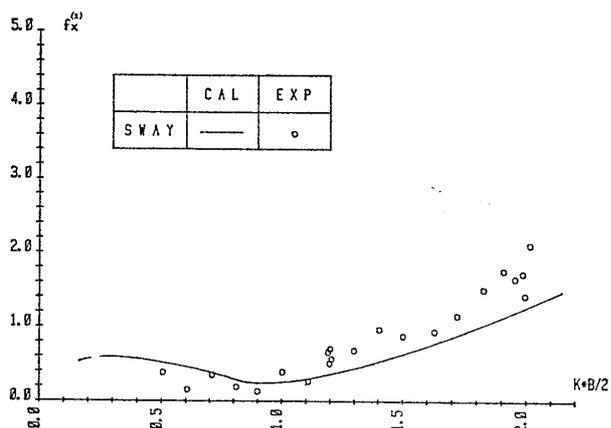
Fig. 11 2nd-order horizontal wave exciting force (circular cylinder)
