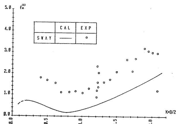
Fig. 13 2nd-order horizontal wave exciting force (rectangular cylinder)
