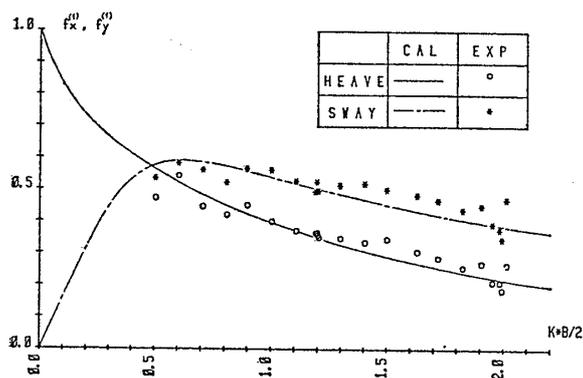
Fig. 8 1st-order wave exciting forces (circular cylinder)
