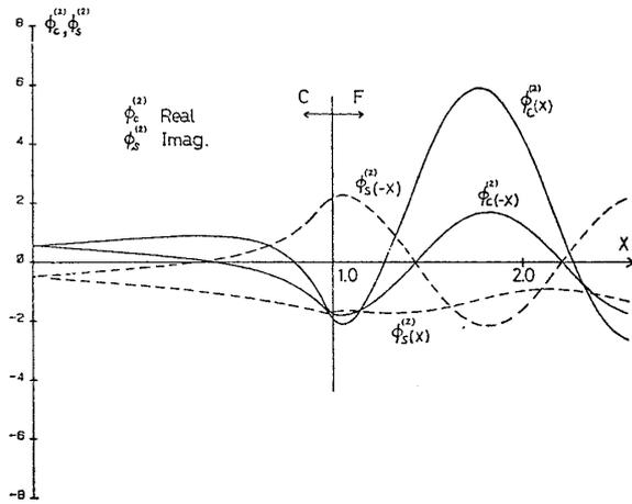
Fig. 6 Distribution of 2nd-order diffraction potential on body and free-surface (circular cylinder,  $Kb=1.0$ )
