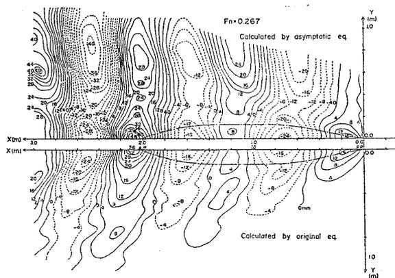
Fig. 4 Calculated wave pattern (Submerged body)  $F_n=0.267$
