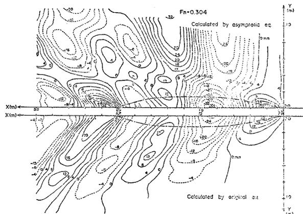
Fig. 5 Calculated wave pattern (Submerged body)  $F_n=0.304$
