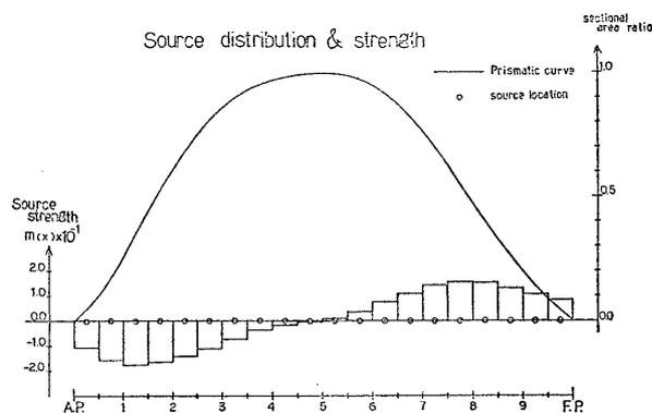
Fig. 3 Source distribution for Series 60
