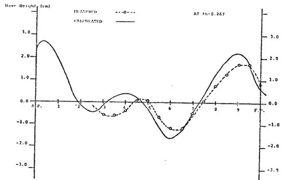
Fig. 12 Calculated and measured wave profile,  $F_n=0.267$
