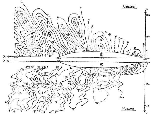
Fig. 11 Calculated and measured wave pattern,  $F_n=0.304$
