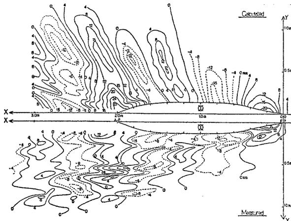
Fig. 10 Calculated and measured wave pattern,  $F_n=0.267$
