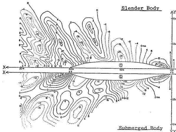
Fig. 9 Calculated wave pattern of Series 60,  $F_n=0.304$
