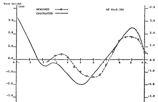
Fig. 13 Calculated and measured wave profile,  $F_n=0.304$
