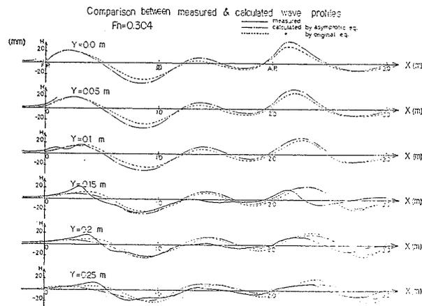
Fig. 7 Wave profiles by the submerged body approximation
