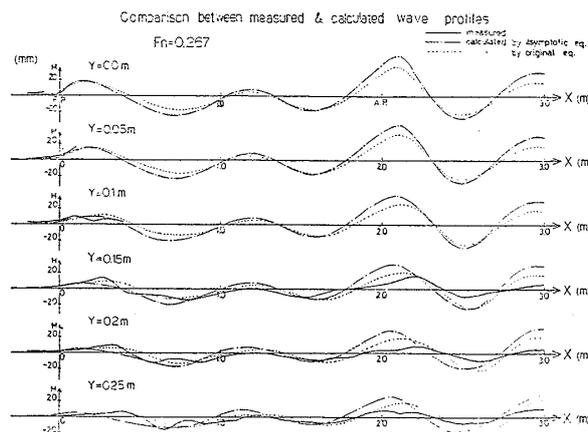
Fig. 6 Wave profiles by the submerged body approximation
