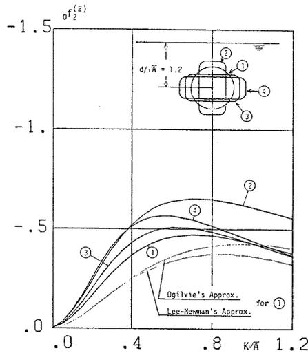
Fig. 19 Vertical steady force of submerged cylinders having various cross-section
