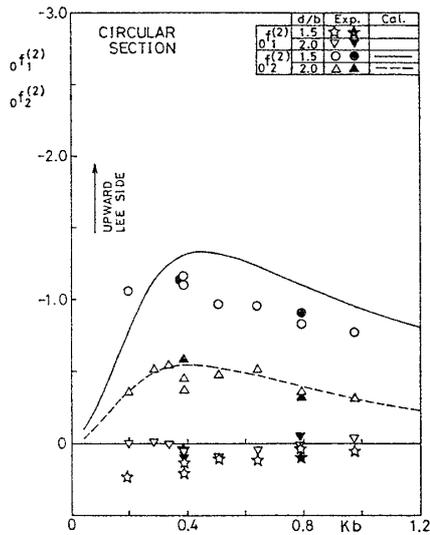
Fig. 9 Drifting force and vertical steady force of submerged circular cylinder
