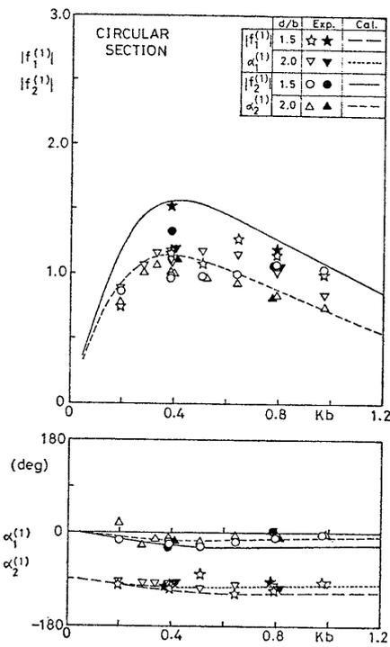
Fig. 7 First-order wave exciting forces of submerged circular cylinder
