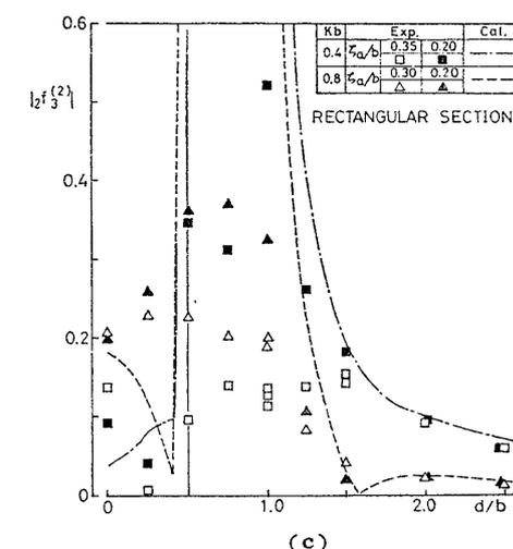
Fig.18 Second-order wave exciting forces and moment of rectangular cylinder as a function of submergence
