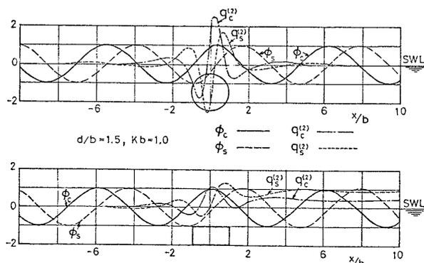
Fig. 2 First-order potential on free-surface and the second-order free-surface condition in diffraction problem ( $Kb=1.0$ )
