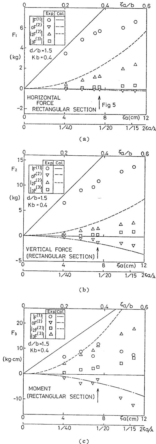
Fig. 6 Each order wave exciting forces and moment as a function of wave amplitude
