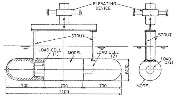
Fig. 4 Arrangement of tests
