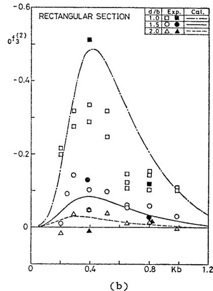
Fig. 10 Drifting force, vertical steady force and steady heeling moment of submerged rectangular cylinder
