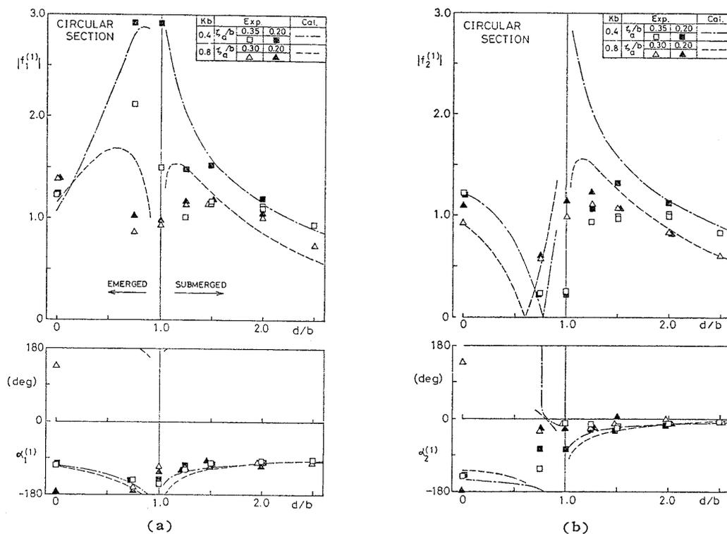
Fig. 13 First-order wave exciting forces of circular cylinder as a function of submergence
