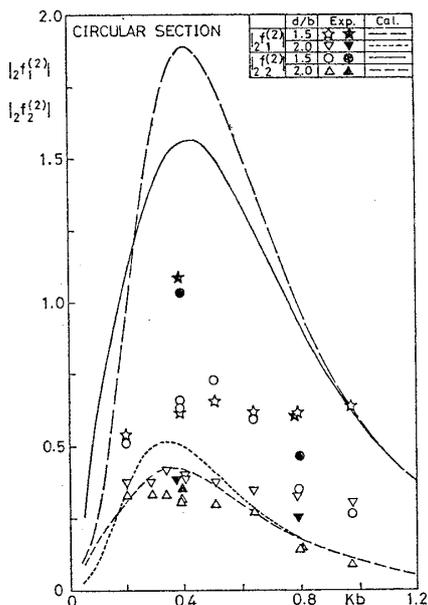
Fig. 11 Second-order wave exciting forces of submerged circular cylinder
