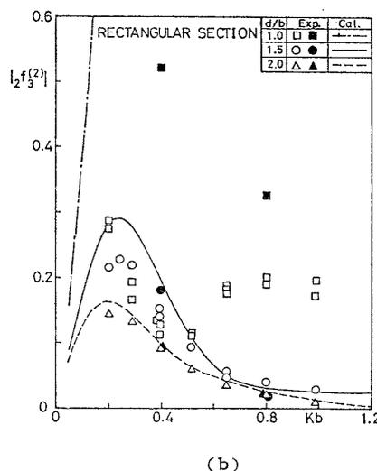
Fig. 12 Second-order wave exciting forces and moment of submerged rectangular cylinder
