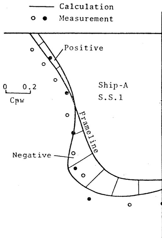
Fig. 9 Comparison of pressure distributions along frame line at S.S.1
