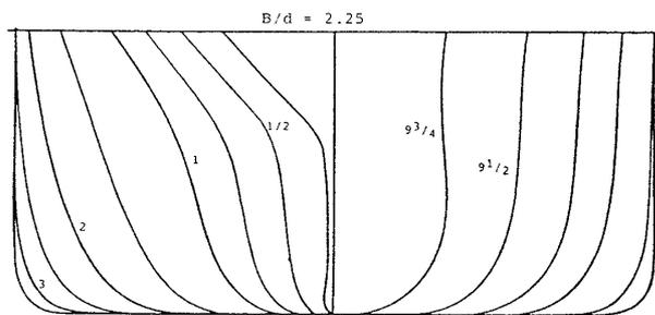
Fig. 8 Body plan of a ship form changed by use of exponential splines
