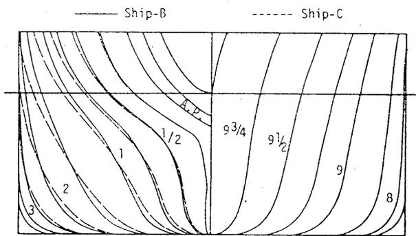
Fig. 11 Body plans of two tanker models
