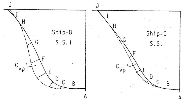
Fig. 12 Distributions of viscous pressure resistance component at S.S.1
