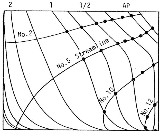
Fig. 2 After-body plan and streamlines of Ship-A
