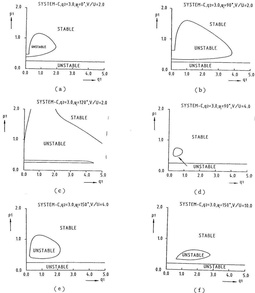
Fig. 6 Stable and unstable zones on the course stability of System-C as function of  $p_1$  and  $q_1$
