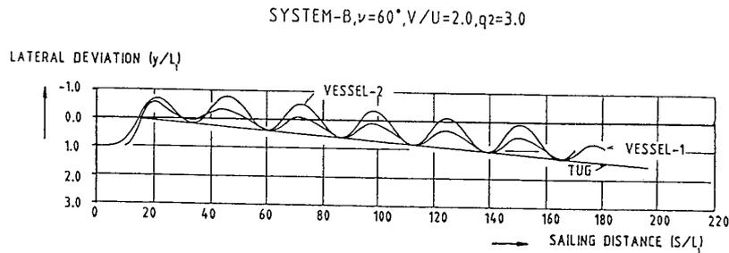
Fig. 9 Trajectory of a tow and two towed vessels in System-B
