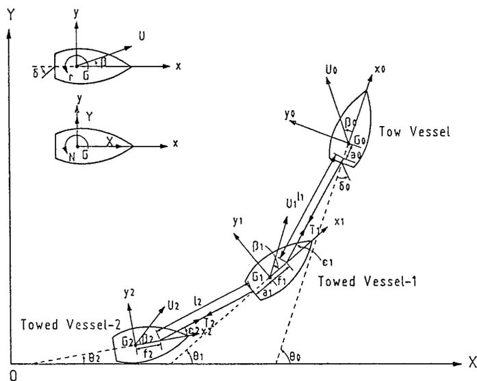
Fig.1 Coordinate systems in tow and towed vessels
