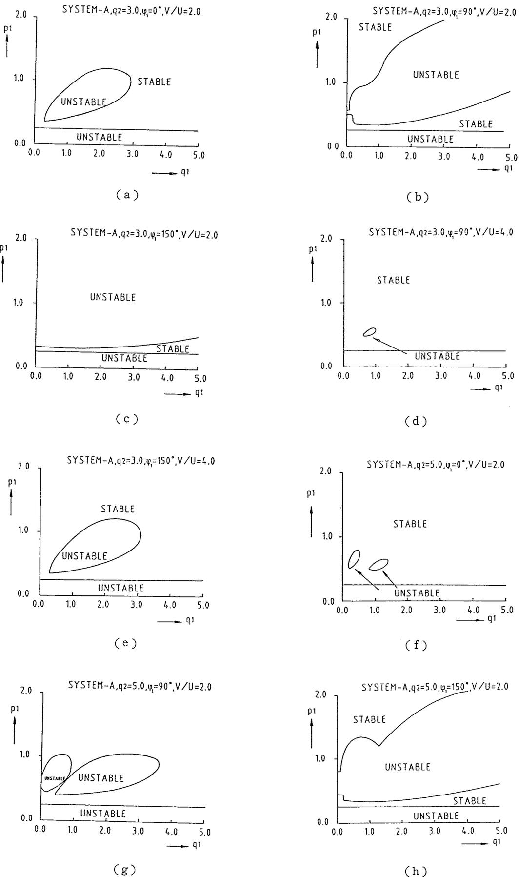
Fig. 4 Stable and unstable zones on the course stability of System-A as function of  $p_1$  and  $q_1$
