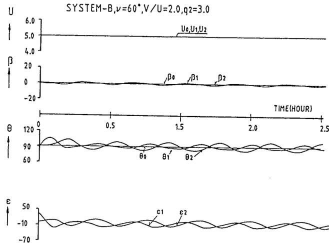
Fig. 10 Time history of the parameters  $U$  (knot),  $\beta$  (degree),  $\theta$  (degree),  $\epsilon$  (degree) of a tow and two towed vessels in System-B
