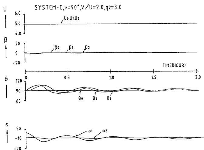
Fig.12 Time history of the parameters  $U$  (knot),  $\beta$  (degree),  $\theta$  (degree),  $\epsilon$  (degree) of a tow and two towed vessels in System-C
