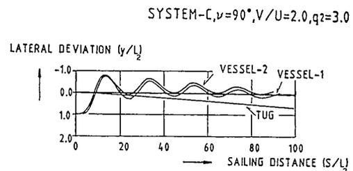
Fig. 11 Trajectory of a tow and two towed vessels in System-C
