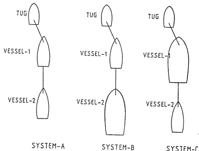
Fig.3 Systems composed of a tow and two towed vessels
