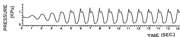
Fig. A1 An example of calculated wall pressure history of a tank with chamfers by harmonic forced excitation
