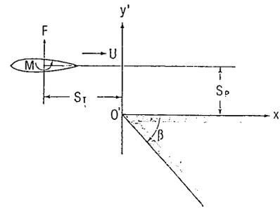
Fig. 2 Coordinate systems for wedge-shaped bank wall
