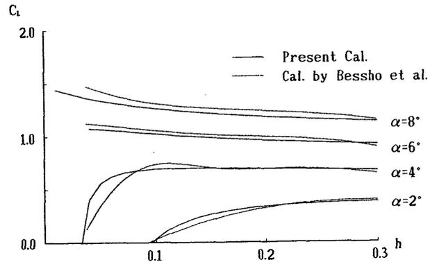
Fig. 6 Comparison of  $C_L$  (NACA 23015)
