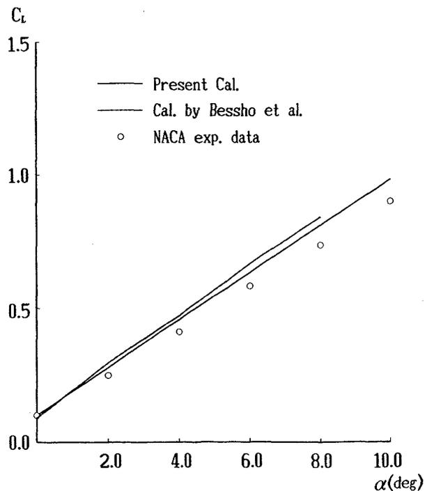
Fig. 4 Comparison of  $C_L$  (NACA 23015)
