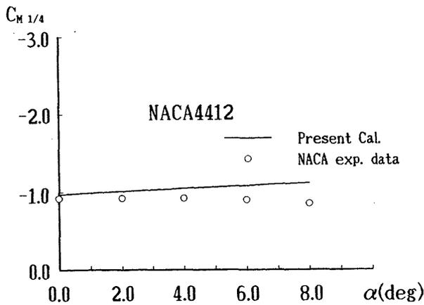
Fig. 5 Comparison of  $C_{M1/4}$  (NACA 0012, NACA 4412)
