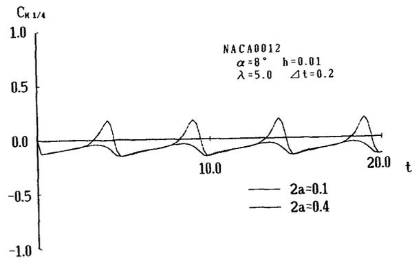
Fig. 20 Comparison of time history  $C_{M1/4}$  (NACA 0012)
