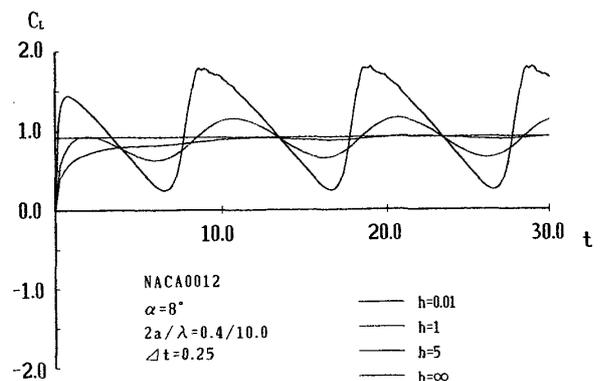
Fig. 19 Comparison of time history  $C_L$  (NACA 0012)
