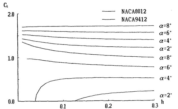
Fig. 8 Comparison of  $C_L$  (NACA 0012 & NACA 9412)
