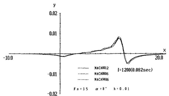
Fig. 12 Comparison of wave profile
