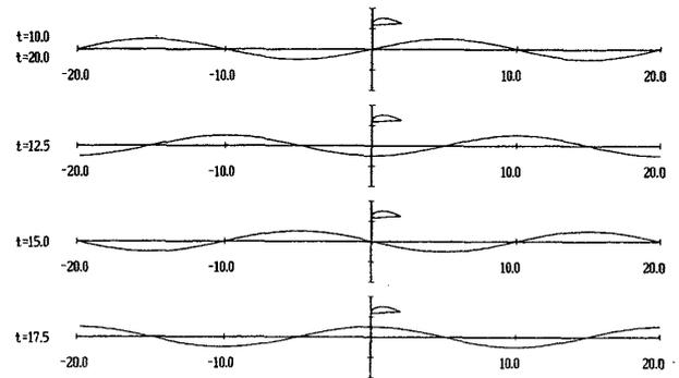
Fig. 17 Positions of WIG on regular wave
