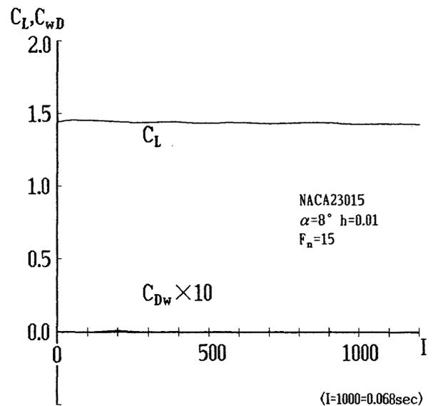
Fig. 11 Time history of  $C_L, C_{DW}$  (NACA 23015)
