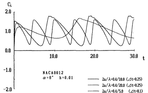
Fig. 18 Comparison of time history  $C_L$  (NACA 0012)
