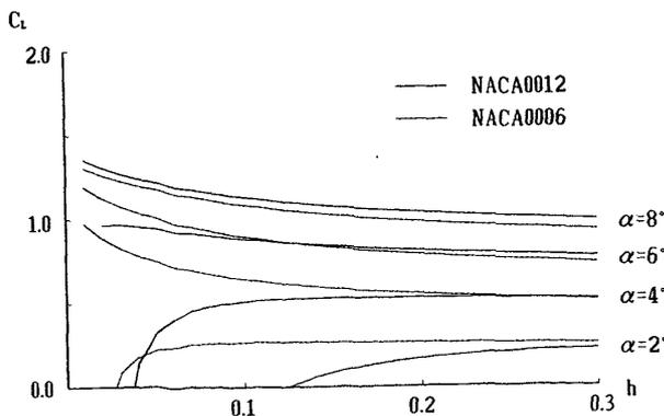
Fig. 7 Comparison of  $C_L$  (NACA 0012 & NACA 0006)
