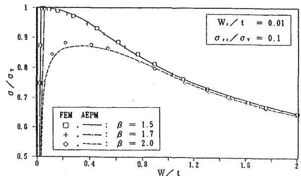
Fig. 16 Stress deflection relationship for the case of thick plates
