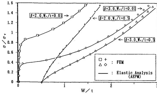
Fig. 8 Comparison of Elastic Analysis with FEM
