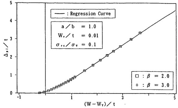
Fig. 10 Relationship between total deflection [ $W - W_v$ ] and plastic deflection  $\Delta_{p1}$  (with residual stress)
