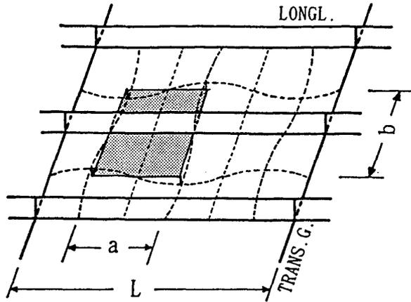
Fig. 2 Local buckling mode
