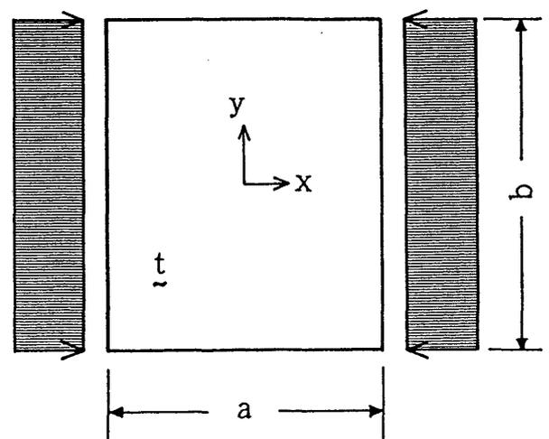
Fig. 1 A rectangular plate subjected to uni-axial compression
