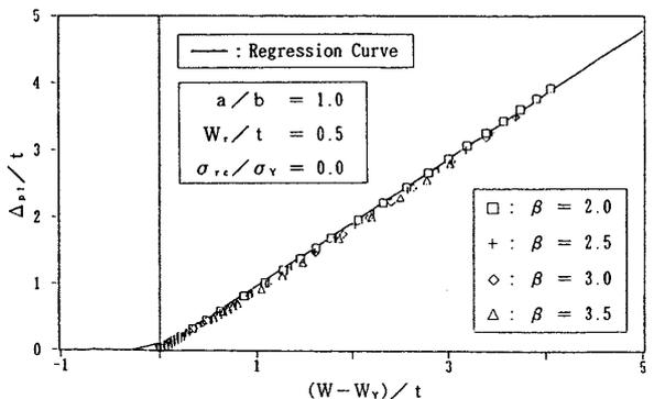
Fig. 11 Relationship between total deflection [ $W - W_v$ ] and plastic deflection  $\Delta_{p1}$  (with initial deflection)
