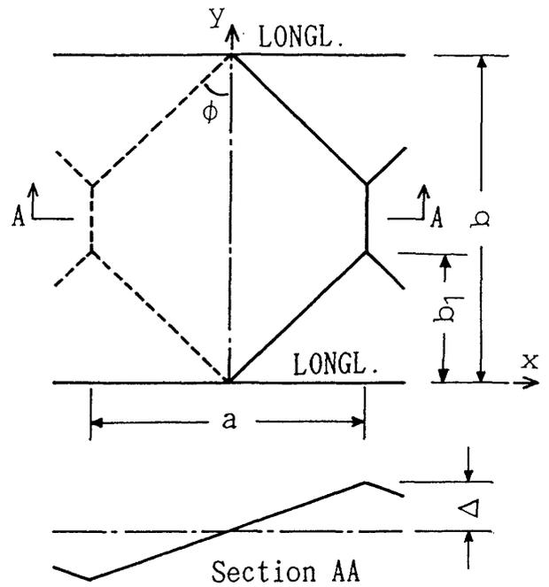
Fig. 4 Hinge lines and plastic deflection
