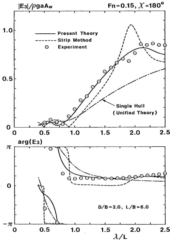
Fig. 8 Heave exciting force on twin Lewis-form ships with  $D/B=2$  at  $F_n=0.15$ , in head wave ( $\chi=180^\circ$ )
