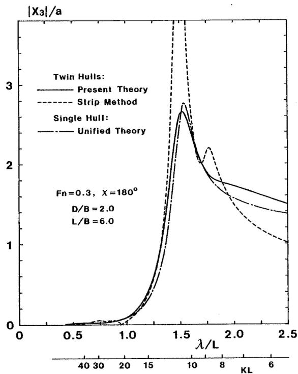
Fig. 14 Modulus of computed heave motion of twin Lewis-form ships with  $D/B=2$  at  $Fn=0.30$ , in head wave
