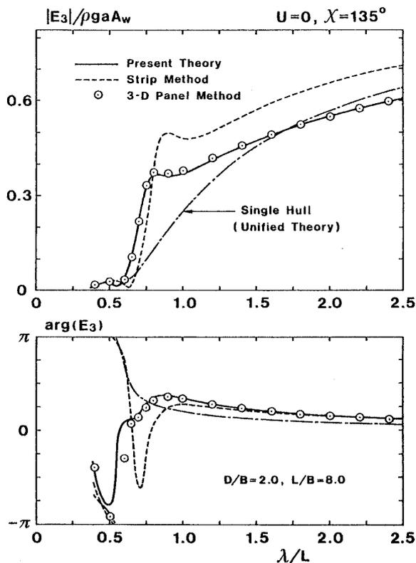
Fig. 4 Heave exciting force on twin half-immersed spheroids with  $B/L=1/8$  and  $D/B=2$  at  $U=0$ , in oblique bow wave ( $\chi=135^\circ$ )
