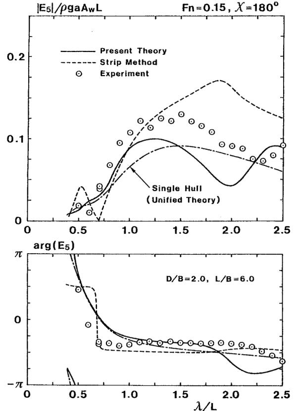
Fig. 9 Pitch exciting moment on twin Lewis-form ships with  $D/B=2$  at  $F_n=0.15$ , in head wave ( $\chi=180^\circ$ )
