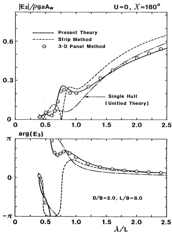
Fig. 2 Heave exciting force on twin half-immersed spheroids with  $B/L=1/8$  and  $D/B=2$  at  $U=0$ , in head wave ( $\chi=180^\circ$ )
