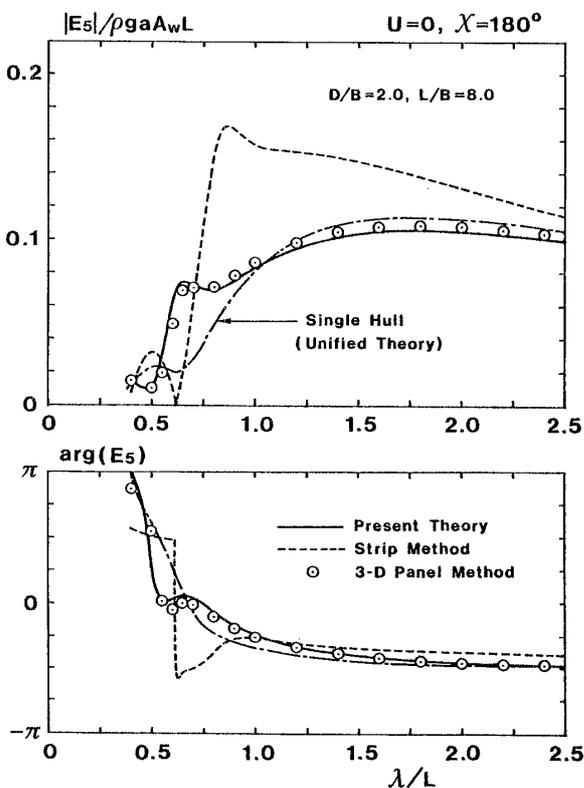
Fig. 3 Pitch exciting moment on twin half-immersed spheroids with  $B/L=1/8$  and  $D/B=2$  at  $U=0$ , in head wave ( $\chi=180^\circ$ )
