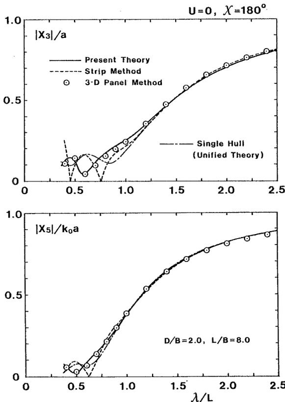
Fig. 6 Modulus of heave and pitch motions of twin half-immersed spheroids with  $B/L=1/8$  and  $D/B=2$  at  $U=0$ , in head wave ( $\chi=180^\circ$ )
