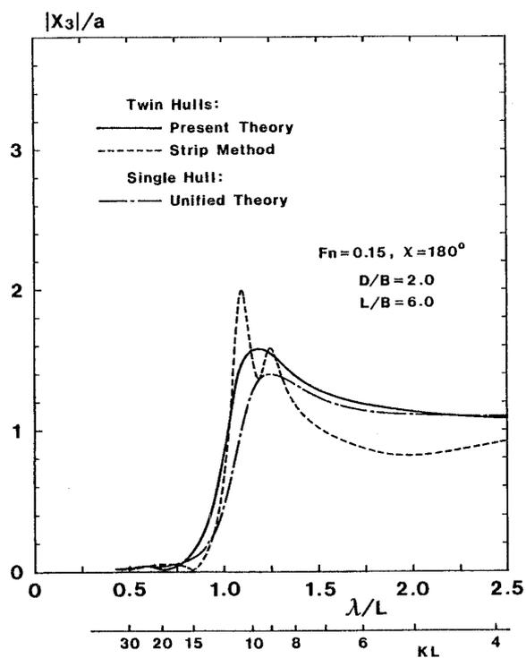
Fig. 12 Modulus of computed heave motion of twin Lewis-form ships with  $D/B=2$  at  $Fn=0.15$ , in head wave
