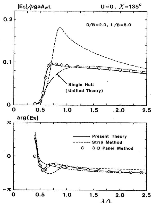
Fig. 5 Pitch exciting moment on twin half-immersed spheroids with  $B/L=1/8$  and  $D/B=2$  at  $U=0$ , in oblique bow wave ( $\chi=135^\circ$ )
