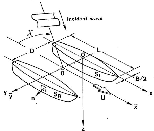
Fig. 1 Coordinate system and notations
