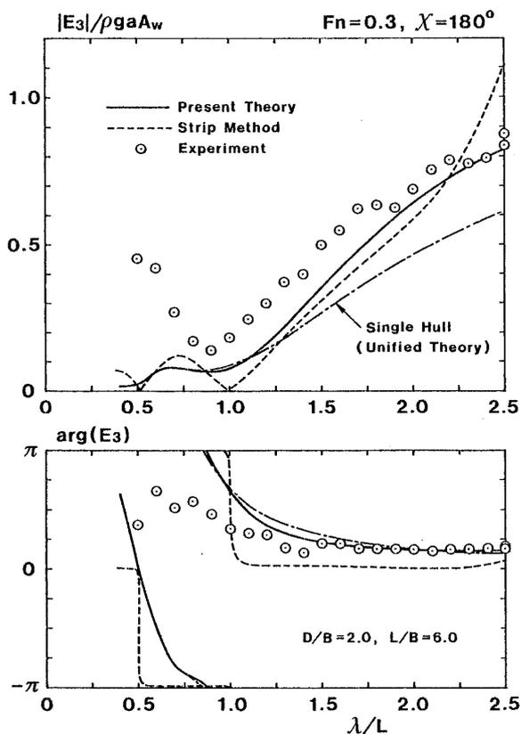
Fig. 10 Heave exciting force on twin Lewis-form ships with  $D/B=2$  at  $Fn=0.30$ , in head wave ( $\chi=180^\circ$ )
