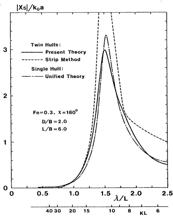
Fig. 15 Modulus of computed pitch motion of twin Lewis-form ships with  $D/B=2$  at  $Fn=0.30$ , in head wave
