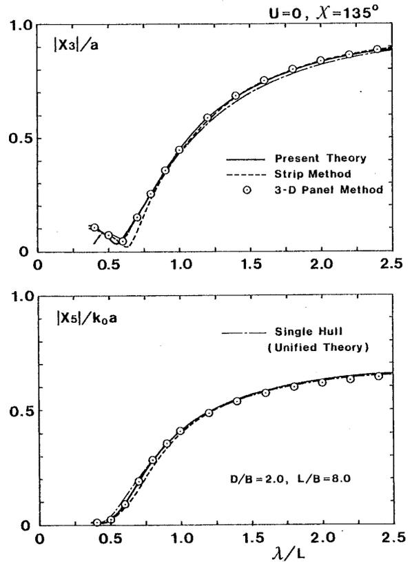
Fig. 7 Modulus of heave and pitch motions of twin half-immersed spheroids with  $B/L=1/8$  and  $D/B=2$  at  $U=0$ , in oblique bow wave ( $\chi=135^\circ$ )
