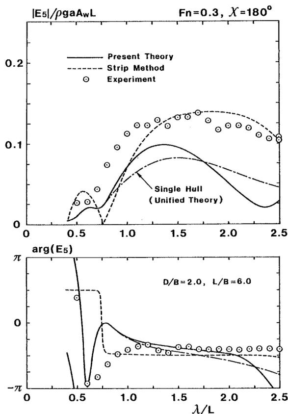
Fig. 11 Pitch exciting moment on twin Lewis-form ships with  $D/B=2$  at  $Fn=0.30$ , in head wave ( $\chi=180^\circ$ )
