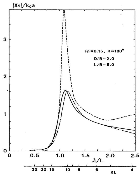
Fig. 13 Modulus of computed pitch motion of twin Lewis-form ships with  $D/B=2$  at  $Fn=0.15$ , in head wave
