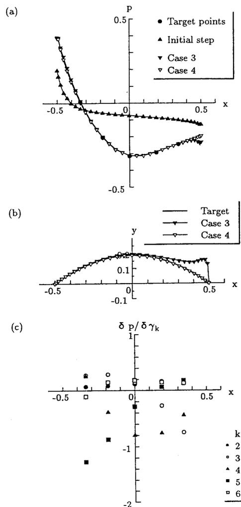
Fig. 5 Case of pressure specified (Case 3 and 4); (a) Distribution of pressure  $p$ ; (b) Comparison of body profiles; (c) Pressure variation in specified point at step  $n=1$
