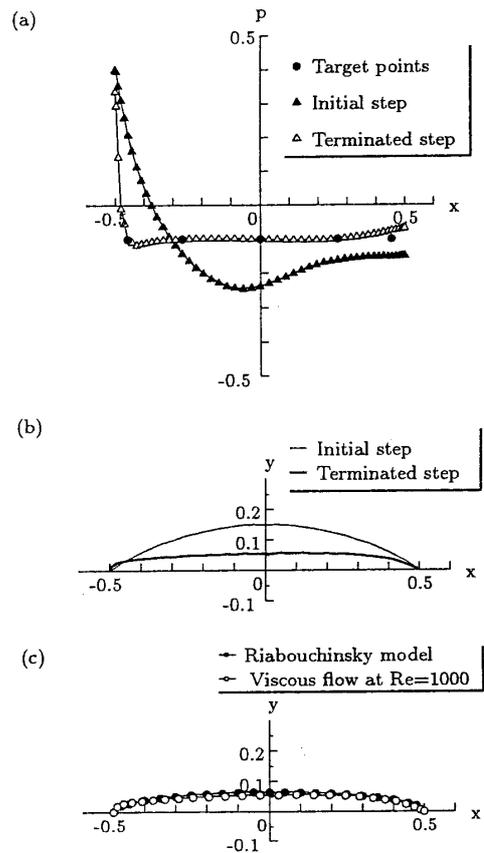
Fig. 10 Constant pressure distribution specified,  $Re=1000$  (Case 4); (a) Distribution of pressure  $p$ ; (b) Comparison of body profiles; (c) Comparison with Riabouchinsky model shape
