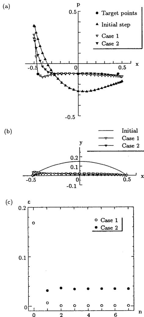
Fig. 8 Constant pressure distribution specified (Case 1 and 2); (a) Distribution of pressure  $p$ ; (b) Comparison of body profiles; (c) Step variation of residual sum of square
