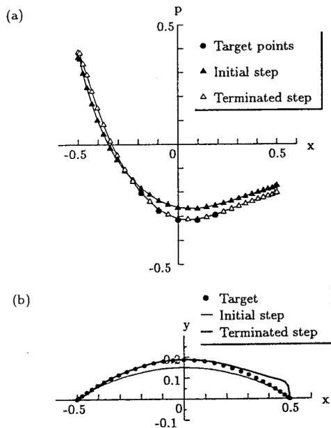
Fig. 3 Case of pressure specified (Case 1); (a) Distribution of pressure  $p$ ; (b) Comparison of body profiles
