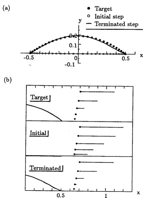
Fig. 6 Case of wake-distribution specified; (a) Comparison of body profiles; (b) Comparison of wake distributions
