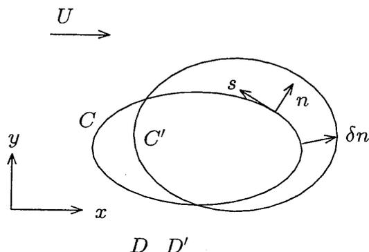
Fig. 1 Boundary deformation
