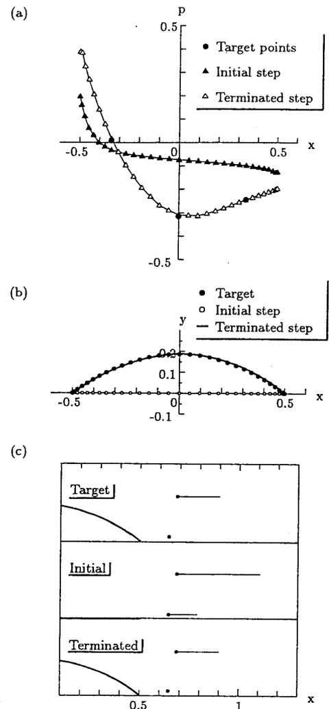
Fig. 7 Case of pressure and wake specified; (a) Distribution of pressure  $p$ ; (b) Comparison of body profiles; (c) Comparison of wake distributions
