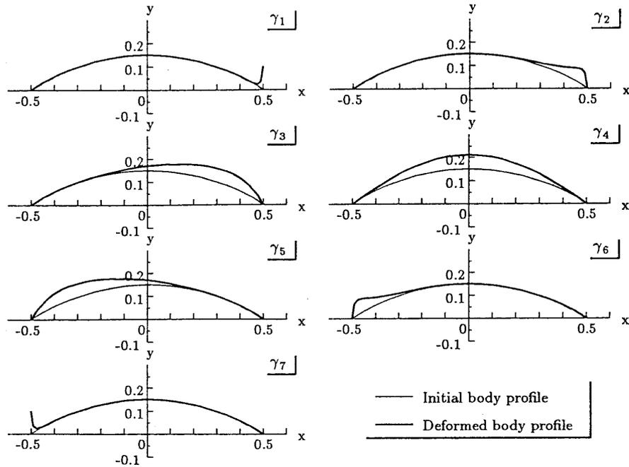
Fig. 2 Body deformation due to  $\gamma_k$  increment by 0.1
