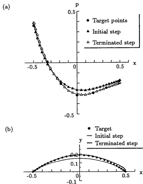
Fig. 4 Case of pressure specified (Case 2); (a) Distribution of pressure  $p$ ; (b) Comparison of body profiles
