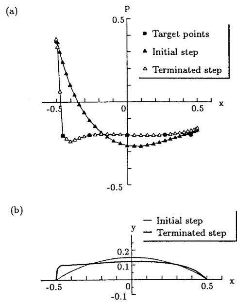
Fig. 9 Constant pressure distribution specified (Case 3); (a) Distribution of pressure  $p$ ; (b) Comparison of body profiles
