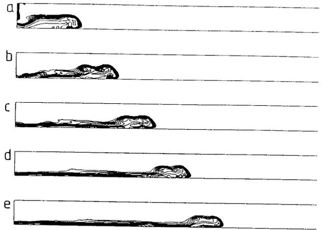
Fig. 5 Development of a gravity current in a lock-exchange flow computed with the no-slip boundary conditions at  $Re=1000$ . Density contours at (a)  $t=4$ , (b)  $t=8$ , (c)  $t=12$ , (d)  $t=16$ , (e)  $t=20$ . The interval of contours is 10% of the initial density difference.
