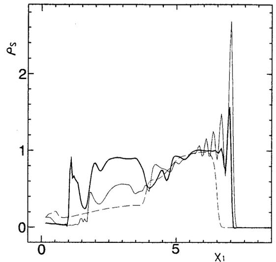
Fig. 1 Comparison of density distributions at the bottom between the difference schemes at  $t=12$ . thick line: QUICK method, thin line: Centred differencing, broken line: Donor-Cell method.
