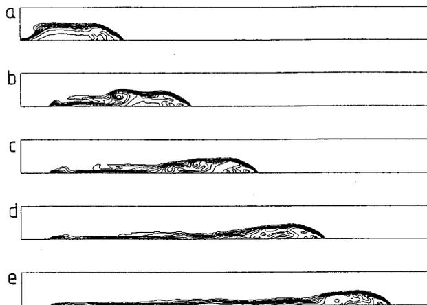
Fig. 2 Development of a gravity current in a lock-exchange flow computed with the free-slip boundary conditions at  $Re=1000$ . Density contours at (a)  $t=4$ , (b)  $t=8$ , (c)  $t=12$ , (d)  $t=16$ , (e)  $t=20$ . The interval of contours is 10% of the initial density difference.
