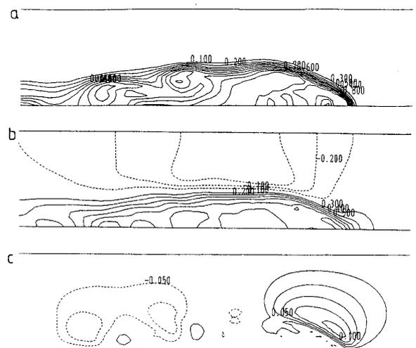
Fig. 3 The flow structure of the head of a gravity current computed with free-slip conditions at  $Re=1000$ . Contours of (a) density, (b) horizontal velocity and (c) vertical velocity at  $t=12$ .
