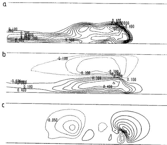
Fig. 6 The flow structure of the head of a gravity current computed with no-slip conditions at  $Re=1000$ . Contours of (a) density, (b) horizontal velocity and (c) vertical velocity at  $t=12$ .
