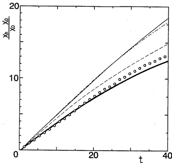
Fig. 7 Position of the front of a gravity current with time.; thin line: QUICK method with free-slip conditions; dash-dotted line: Centred differencing with free-slip; broken line: Donor-cell method with free-slip; thick line: QUICK method with no-slip conditions; circles: experiment.
