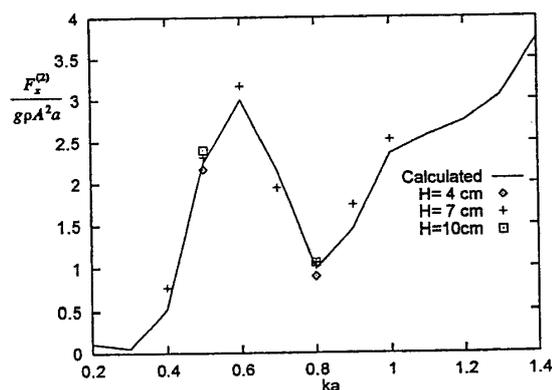
Fig. 9 Comparison of wave drift force on four restrained cylinders at  $Fr=0.05$ .
