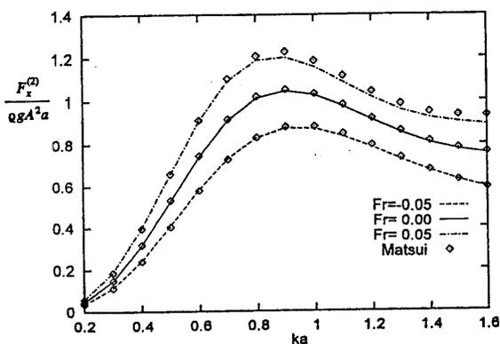
Fig. 7 Second order mean drift forces on a uniform cylinder of radius  $a$  in a water depth of  $h/a=1$ .
