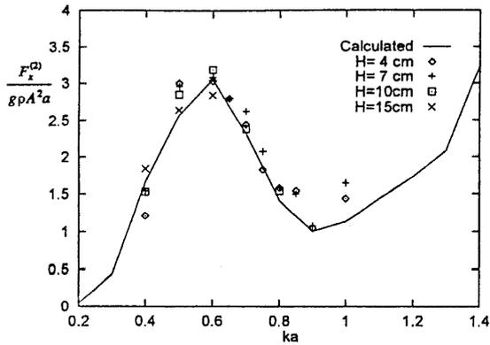
Fig. 12 Comparison of wave drift force on four freely moving cylinders at  $Fr=0.05$ .
