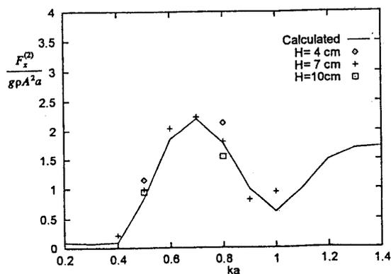
Fig. 11 Comparison of wave drift force on four restrained cylinders at  $Fr=-0.05$ .
