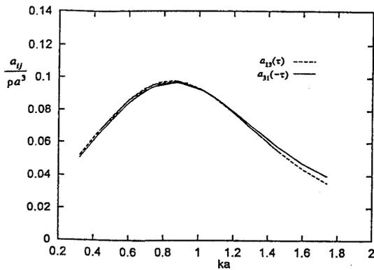
Fig. 3 Cross coupling surge-heave added mass of an hemisphere of radius  $a$  in a water depth of  $h/a=2$
