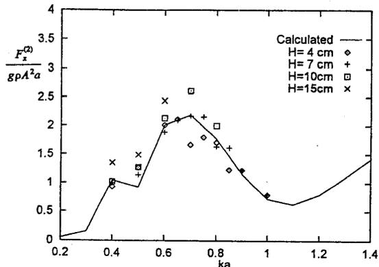
Fig. 14 Comparison of wave drift force on four freely moving cylinders at  $Fr=-0.05$ .
