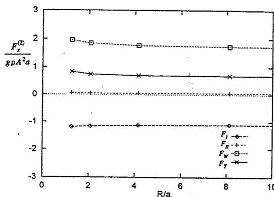
Fig. 1 Examination on the convergence with radius of the mesh on the free surface for second order drift force on a truncated cylinder at  $Fr = -0.10$  and  $ka = 1.5$ .
