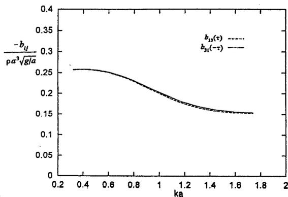
Fig. 4 Cross coupling surge-heave damping coefficients of an hemisphere of radius  $a$  in a water depth of  $h/a=2$
