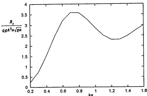
Fig. 8 Wave damping of a uniform cylinder of radius  $a$  in a water depth of  $h/a=1$ , obtained by numerical differentiation of the mean drift forces at  $Fr = +/- 0.05$ .
