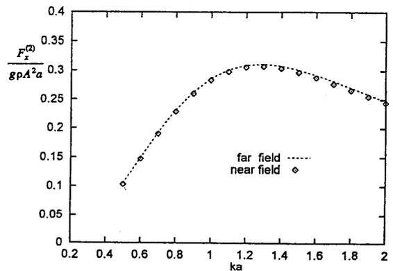
Fig. 5 Comparison of second order drift force on the hemisphere by the near and far field methods
