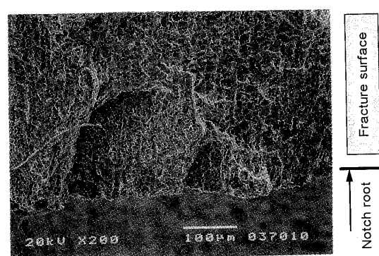
Fig. 12 Grown-up pits during crack growth in H_2SO_4 at pH 4 ( K_t=2.0 , \Delta S=300 MPa, N_c=6.44 \times 10^4 , N_f=7.08 \times 10^4 )
