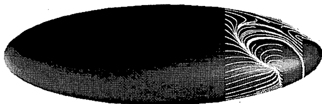
Fig.1b Particles are released around the first separation line.
