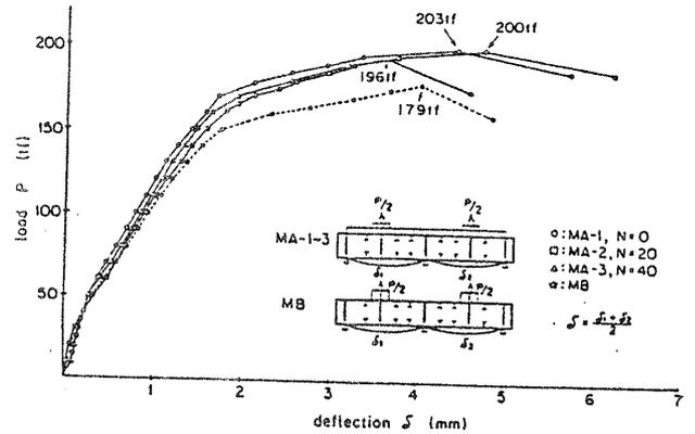
Fig. 4 Measured load-deflection curves
