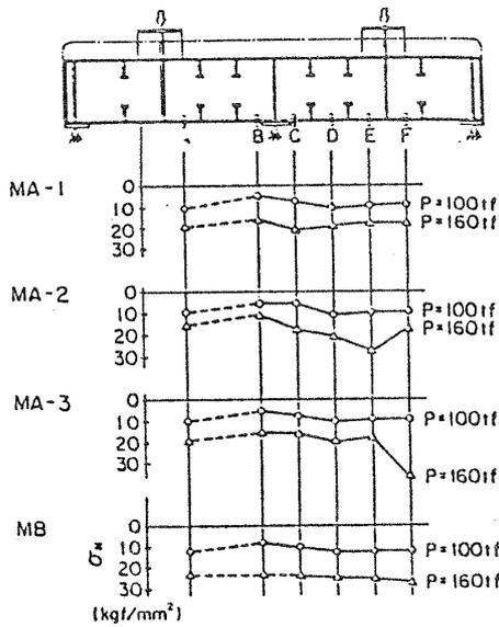
Fig. 8 Measured load-axial stresses of steel plates relation
