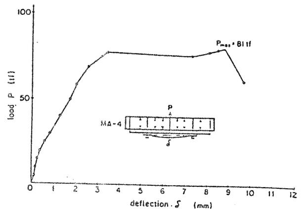
Fig. 5 Measured load-deflection curves (MA-4)
