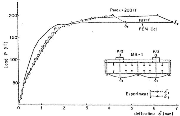
Fig. 10 Comparison of load-deflection curves (MA-1)
