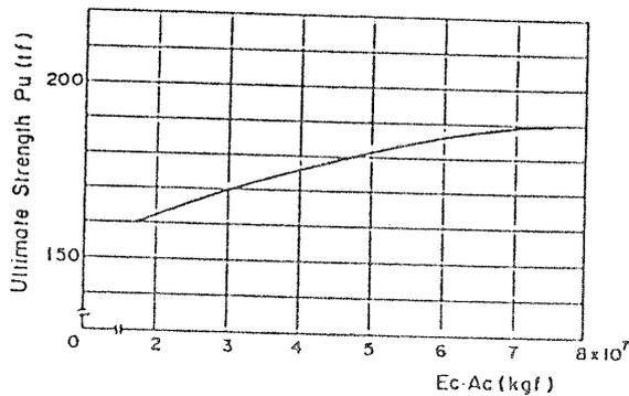
Fig. 16 Relation between ultimate strength and axial stiffness
