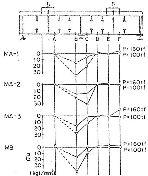
Fig. 9 Measured bending stresses of steel plates
