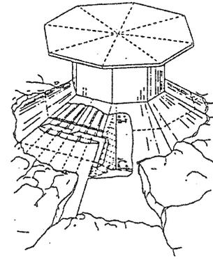
Fig. 1 Ice-resistant wall of Arctic offshore structure
