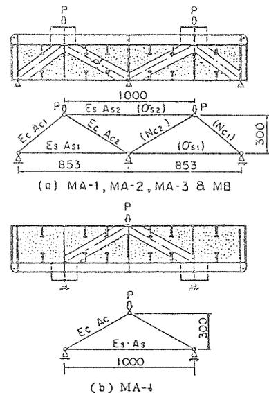
Fig. 14 Simplified model for ultimate strength analysis
