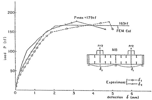
Fig. 12 Comparison of load-deflection curves (MB)
