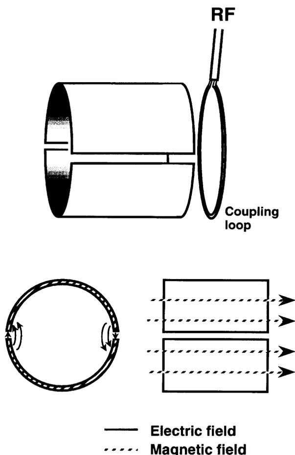
**Fig. 2.** Loop-gap resonator with two-gaps. Matching of the RF line to the resonator is performed by mechanically changing the distance between the coupling loop and the resonator loop.
