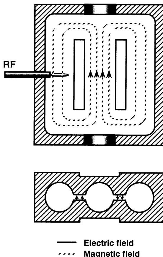
**Fig. 3.** Re-entrant resonator. Matching of the RF line to the resonator is performed by rotating the coupling loop.
