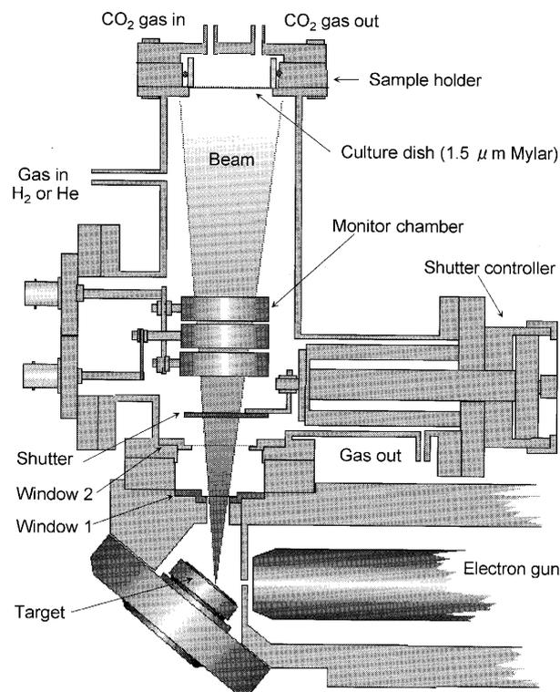
Fig. 1. Cross sectional view of the X-ray tube.
