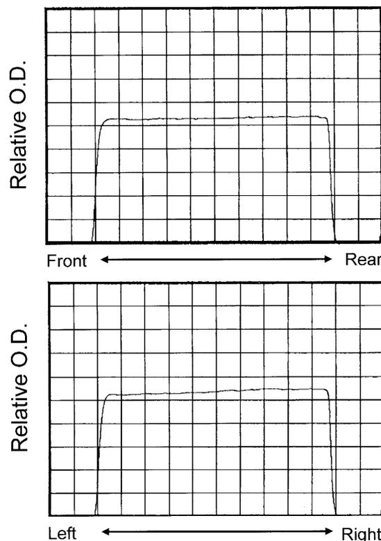
Fig. 2. The dose uniformity at the flight tube window as measured by optical density of photographic films exposed to Al<sub>K</sub> X-rays.
