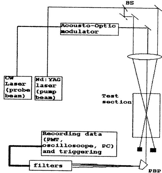
Fig. 2. Optical set up for LITA experiment
