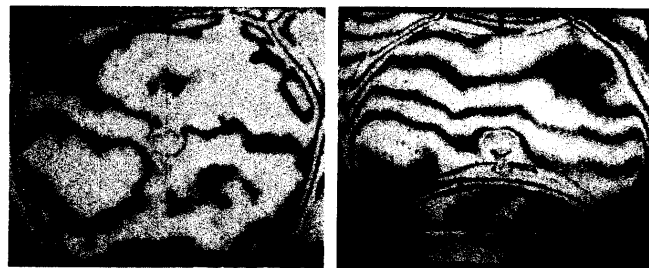
Fig.2 Visualization of propagating blast wave: (Left) Normal condition; (Right) Temperature gradient:
