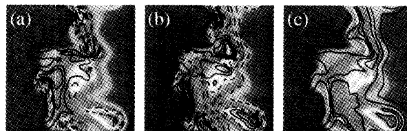
Fig. 7 Contour line of convection term (a), diffusion term (b) and reaction term (c) of H, and distributions of heat release rate.
