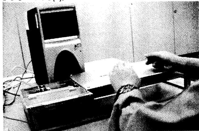
Fig.14 Input device and operation of guidewire simulator
