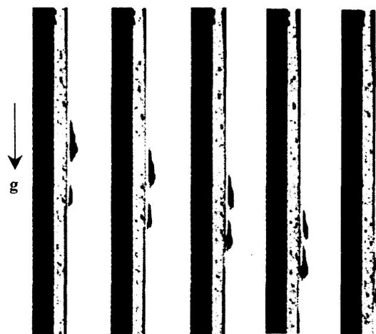
Fig.1 Collision of two solitons (film flow).
