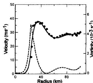
Fig.1 Radial profiles of basic flow: tangential flow (solid line) and vertical vorticity (dotted line).
