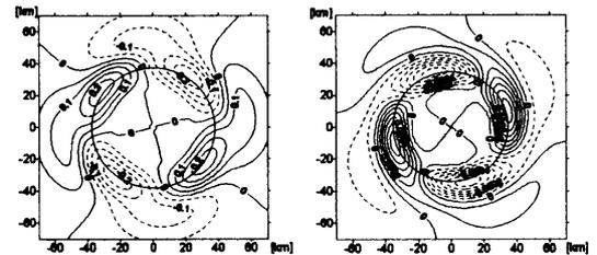
Fig.3 Eigenfunctions of streamfunction and vertical velocity for the most unstable mode: (left) streamfunction for  $m=2, a=0.005$  and (right) vertical velocity for  $m=2, a=0.005$ .
