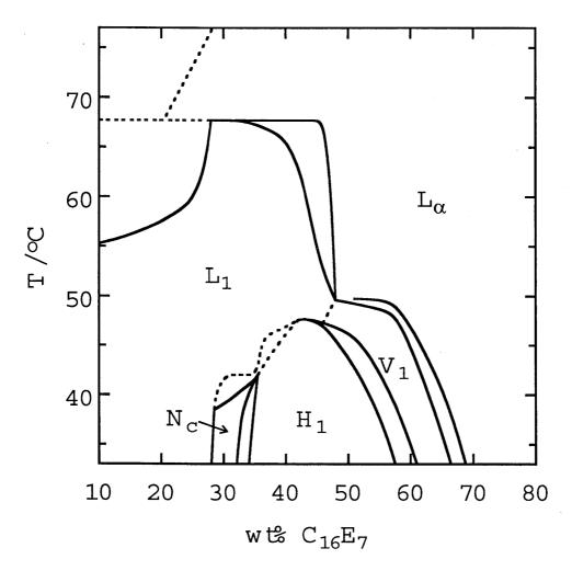
Figure 1: Phase diagram of the  $C_{16}E_7/water$  system.  $L_{\alpha}$ , lamellar phase;  $L_1$ , isotropic micellar phase;  $L_3$ , sponge phase;  $V_1$ , cubic phase;  $H_1$ , hexagonal phase.
