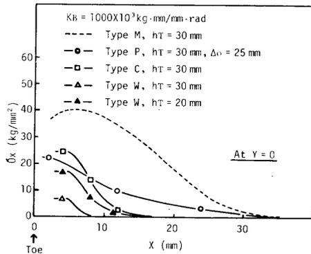
Fig. 9 Transverse welding residual stress distributions measured experimentally
