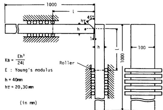
Fig. 1 Apparatus for Corner Joint Weld Cracking Test (CJC-test)
