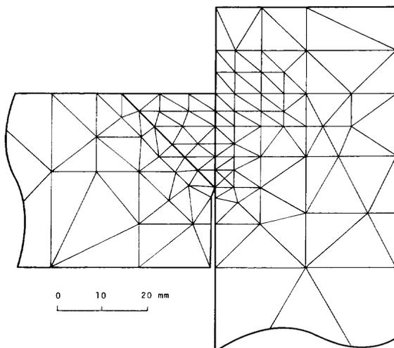
Fig. 6 Mesh division for elastic-plastic analysis
