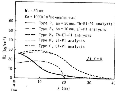
Fig. 10 Transverse welding residual stress distributions analyzed theoretically
