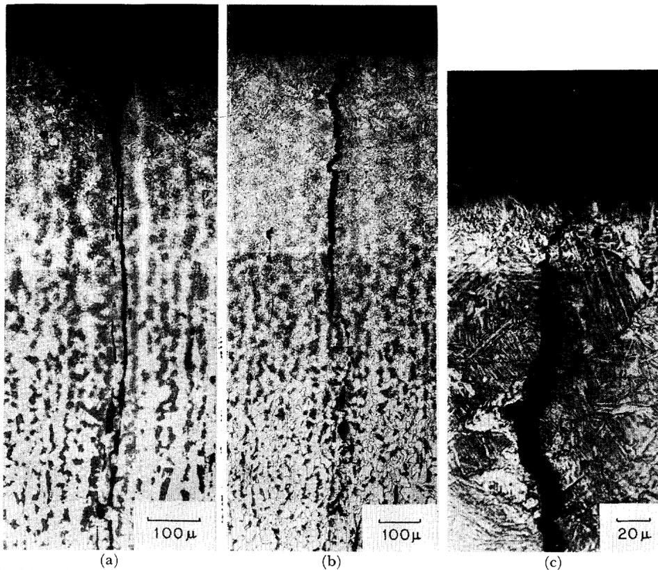
Photo. 2 Microphotographs of lamellar tearing (Type G,  $h_T=30$  mm, (c); magnified photograph of photo. (b))
