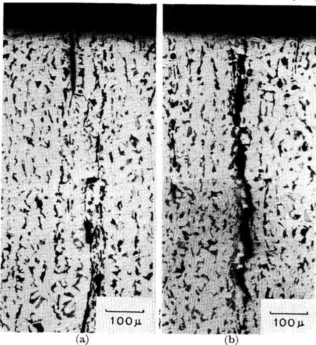
Photo. 3 Microphotographs of lamellar tearing (Type M,  $h_T=30$  mm)
