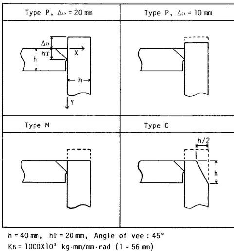
Fig. 5 Shapes of grooves for elastic-plastic analysis
