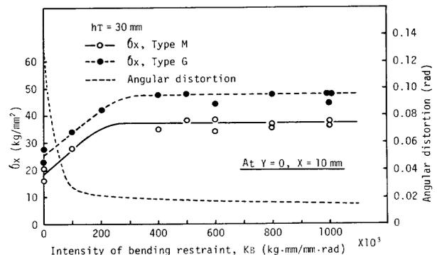
Fig. 8 Effects of intensity of bending restraint on transverse welding residual stress and angular distortion
