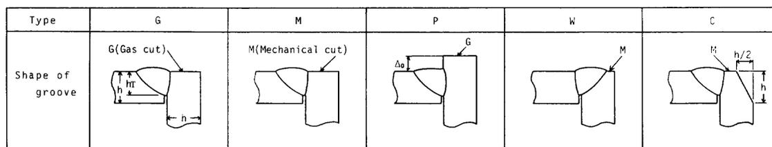
$h = 40 \text{ mm}$ ,  $h_T = 20, 30 \text{ mm}$ , Angle of vee:  $45^\circ$
