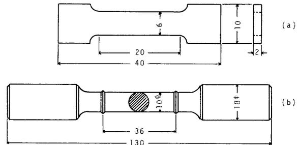
Fig. 11 Test specimens for tension test
