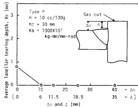
Fig. 4 Relation between lamellar tearing and  $\Delta_0$  ( $\Delta$ )
