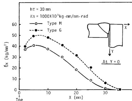
Fig. 7 Transverse welding residual stress distributions measured experimentally
