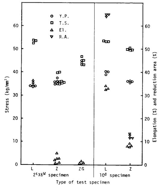
Fig. 12 Results of tension tests
