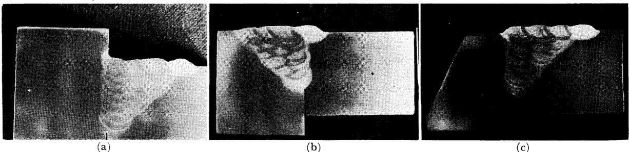
Photo. 4 Macrophotographs of weldments ( $h_T=30$  mm) (a) Type P, (b) Type W, (c) Type C
