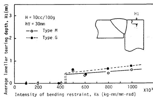
Fig. 3 Relation between lamellar tearing and intensity of bending restraint
