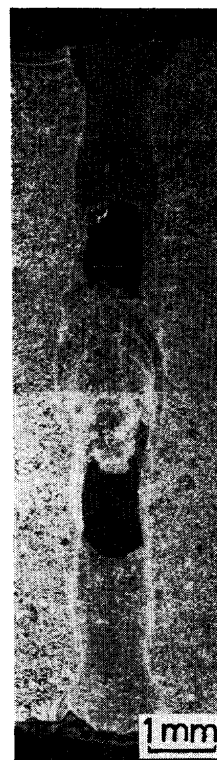
Photo. 14 View of pore at welded zone, 150 kv, 11 mA, 1000 mm/min, a_b^* = 0.95 , 18% porosity
