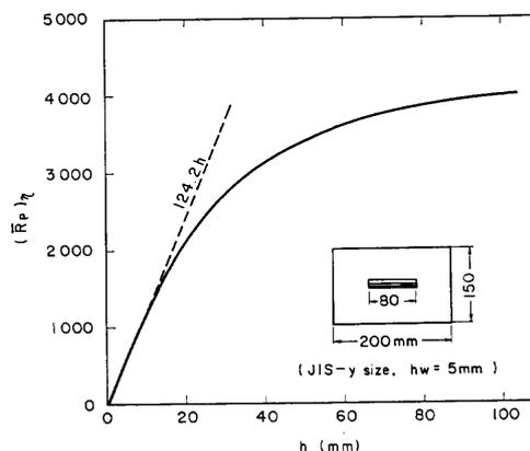
Fig. 2 Effective intensity of restraint (mean value) for the JIS-y test specimen (Ueda, and Kim).
