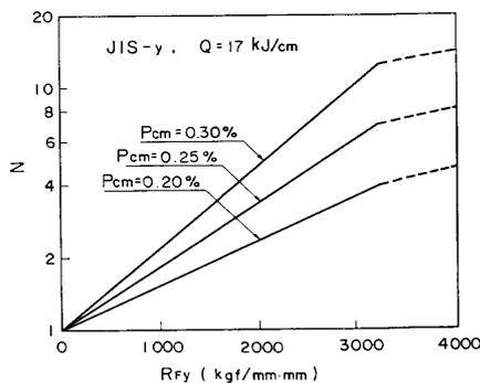
Fig. 5 Ratio  $N$  of hydrogen accumulation.
