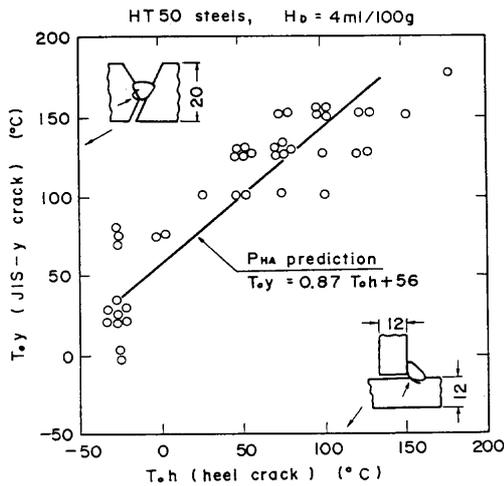
Fig. 11 Comparison of critical preheating temperature for heel cracking versus JIS-y root cracking (HT50 steels, test data by Tanaka and Kitada).
