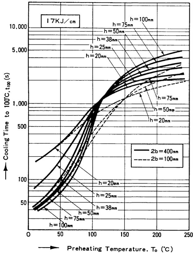
Fig. 14(g) Relation of cooling time to preheating temperature (17 kJ/cm)
