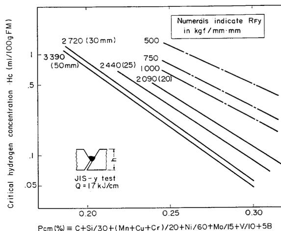
Fig. 3 Relationship between critical hydrogen concentration  $H_c$ , carbon equivalent P<sub>cm</sub> and intensity of restraint  $R_{Fy}$  in JIS-y test ( $Q = 17 \text{ kJ/cm}$ ).
