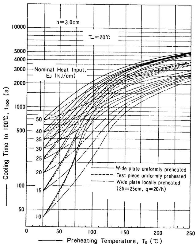
Fig. 14(c) Cooling time to 100°C ( $h=3.0$  cm)
