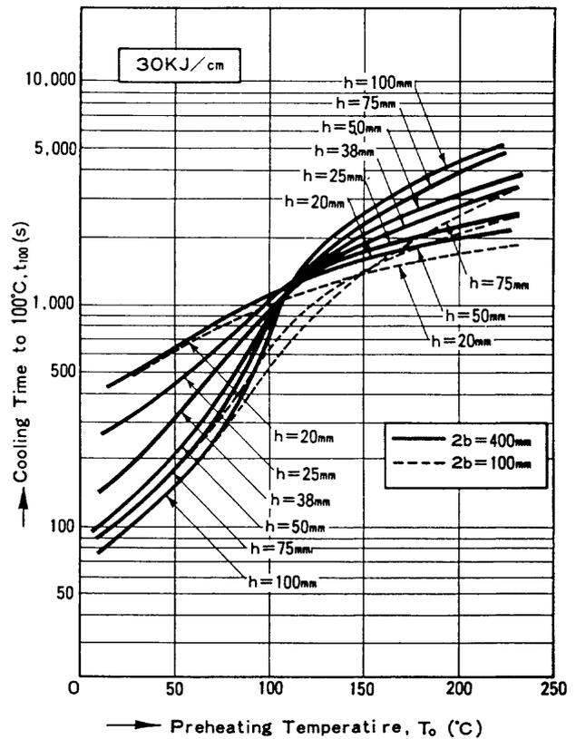
Fig. 14(h) Relation of cooling time to preheating temperature (30 kJ/cm)
