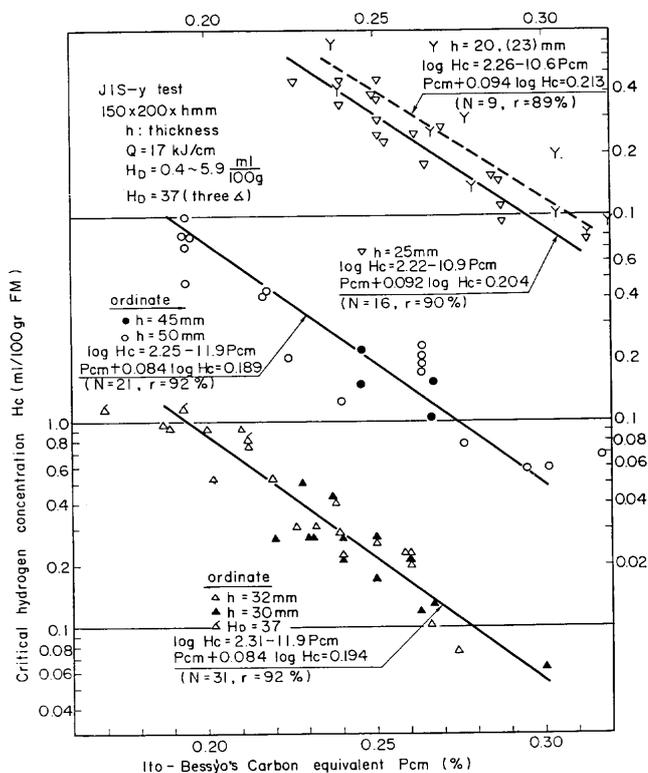
Fig. 1 Effects of P<sub>cm</sub> and plate thickness on the critical hydrogen concentration  $H_c$  in the JIS-y test, including three 32 mm steels with high cellulose electrode.
