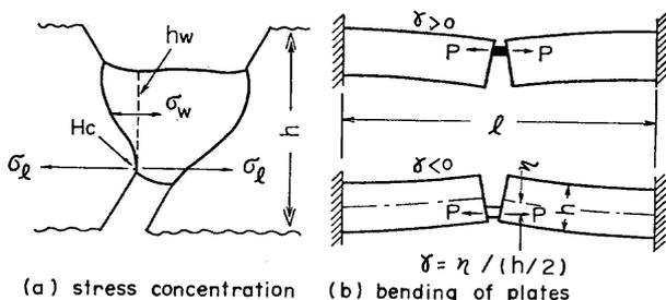
Fig. 12 Notations for calculating  $R_{Fy}$ .
