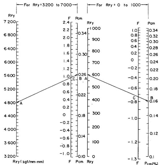
Fig. 13(b) Nomograph to calculate  $F$  for  $R_{Fy}$  ranges of  $0$  to  $1,000$  and  $3,200$  to  $7,000 \text{ kgf/mm}\cdot\text{mm}$ .
