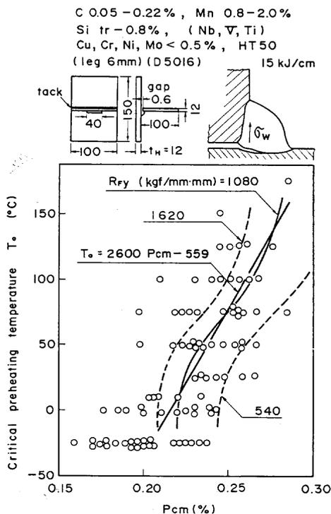
Fig. 10 Critical preheating temperature to avoid heel cracking in HT50 steels of C-Mn-(X) type (test data by Tanaka Kitada) ( $t_H = 12$  mm,  $H_D = 4.0$  ml/100 g JIS).
