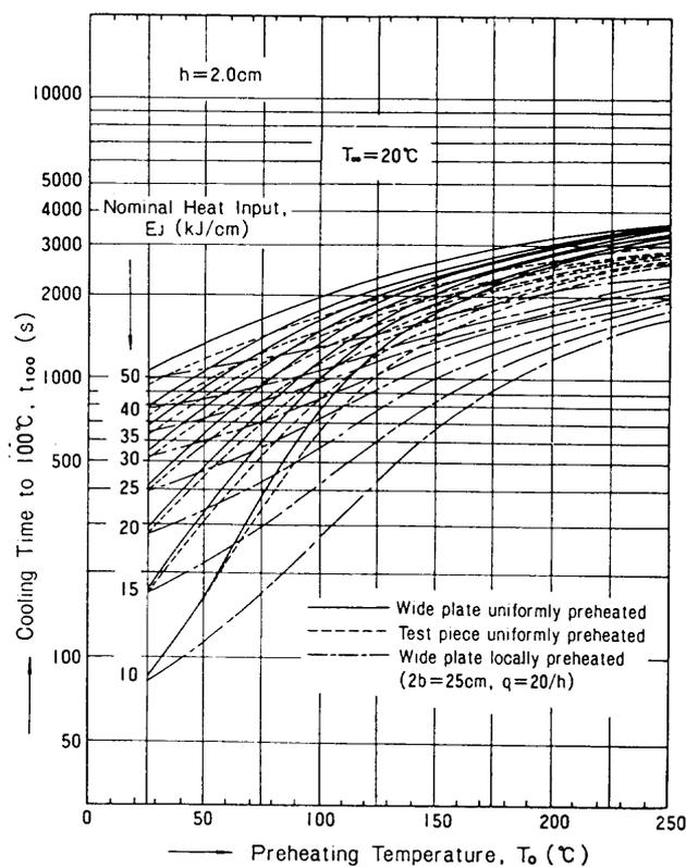
Fig. 14(b) Cooling time to 100°C ( $h=2.0$  cm)
