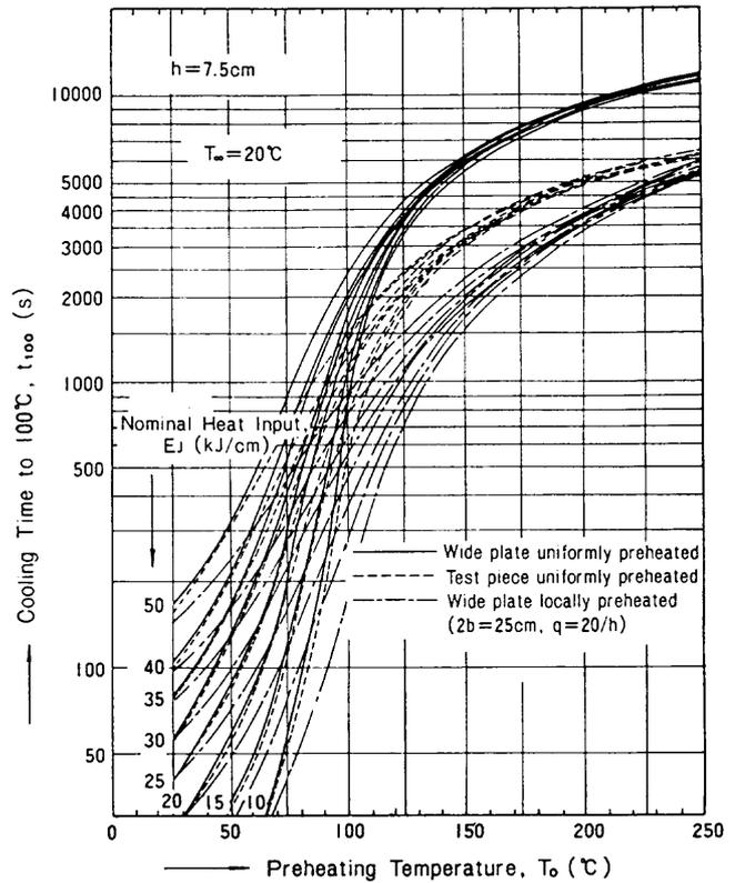
Fig. 14(f) Cooling time to 100°C ( $h=7.5$  cm)
