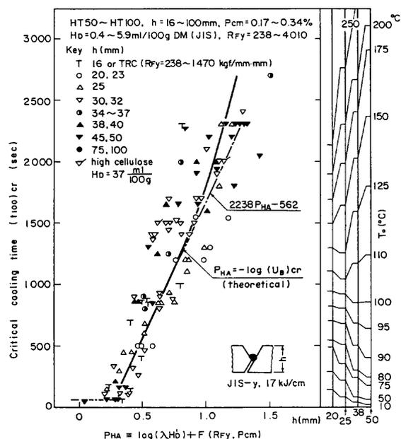
Fig. 6 Relationship between critical cooling time  $(t_{100})cr$  and cracking parameter  $P_{HA}$  for the JIS-y test with weld heat input of 17 kJ/cm.
