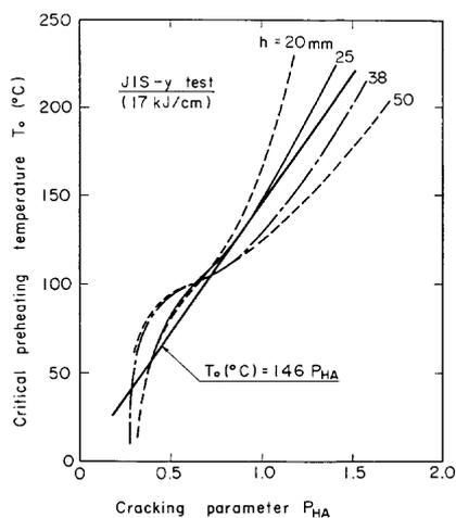
Fig. 8. Relationship between critical preheating temperature  $T_0$ , cracking parameter  $P_{HA}$  and specimen thickness  $h$  in the JIS-y test.
