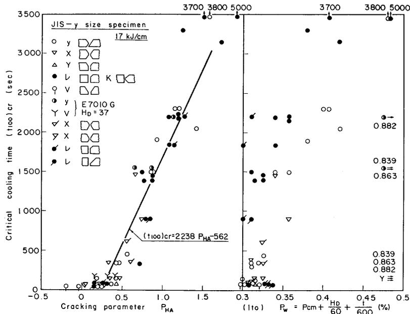
Fig. 9 Correlation between critical cooling time and cracking parameter  $P_{HA}$  or  $P_w$  (Ito-Bessyo) for various groove shapes and weld locations (root cracking in the HAZ in the JIS-y size specimens, 17 kJ/cm).
