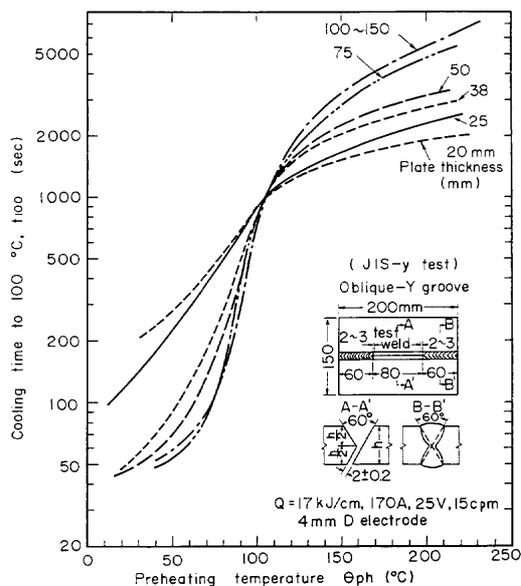
Fig. 7 Relationship between cooling time to 100°C, preheating temperature and plate thickness for the JIS-y test specimens ( $Q=17$  kJ/cm) (JSSC).
