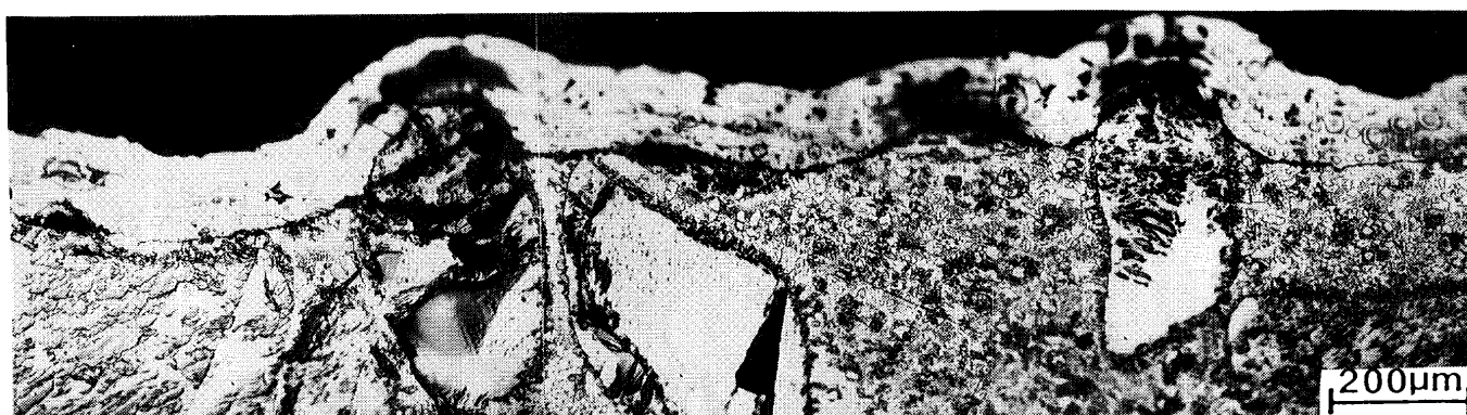
Fig. 7 Cross section of wear surface, (base alloy powder C/V-C).
