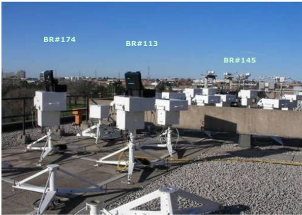
Photo. 1 Intercomparison between MSC and JMA standard Brewer Spectrophotometers on the roof top at MSC in 2010.
