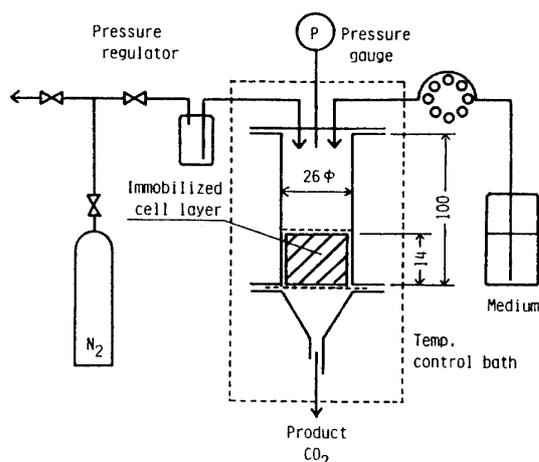
Fig. 1. Immobilized cell system with forced substrate supply.
