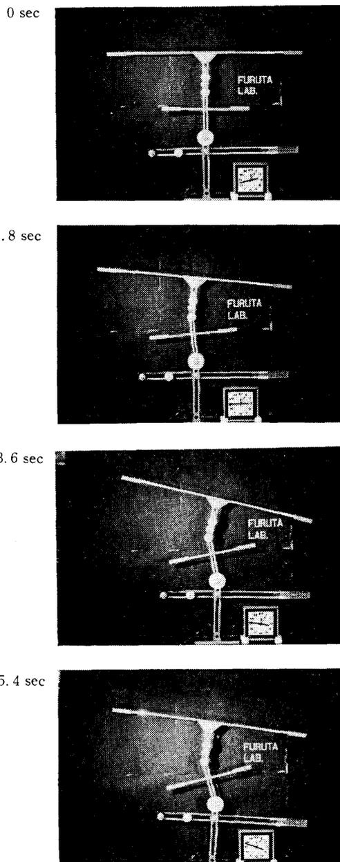
Photo.1 Attitude control of triple inverted pendulum
