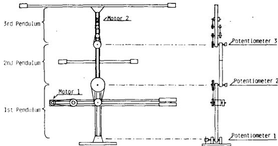
Fig. 1 Triple inverted pendulum
