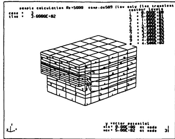
図 2-5 Stream Function  $\Phi$ , at Re=5000 Transient Case
