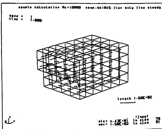
図 2-4 Flow Velocity at Re=10000 Steady Case
