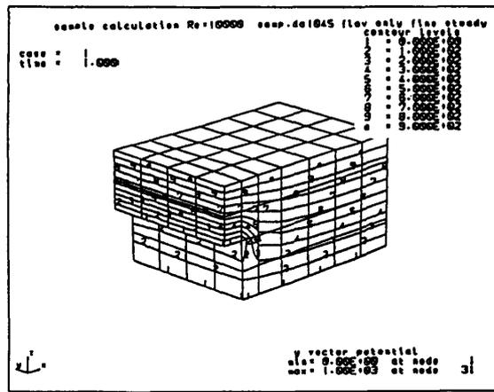
図 2-3 Stream Function  $\Phi$ , at Re=10000 Steady Case
