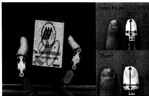
Fig. 2 Novel robot hand with human mimic fingertip. The fingertip parts are molded using a cast which is made by human finger.
