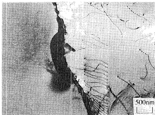
Fig.5 TEM structure in as-welded fusion zone.
