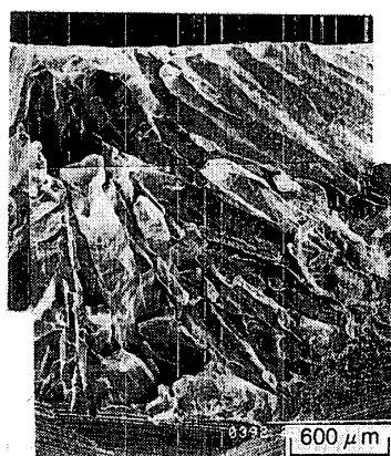
Fig.5 General appearance of crack surface
