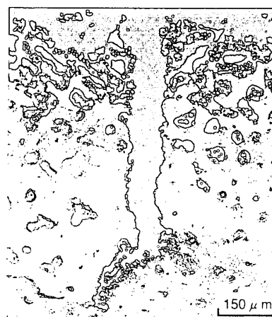
Fig.2 SEM structure of liquation crack at HAZ
