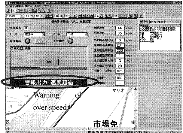
Fig.10 Example of monitoring system for over speed detection.
