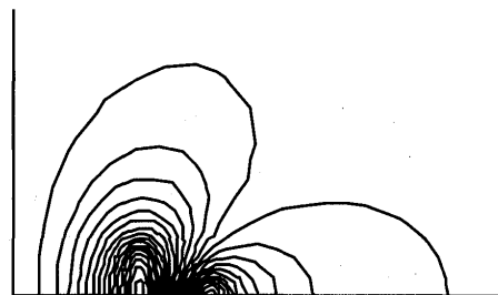
Fig. 2. The optimized field contours of the SMES
