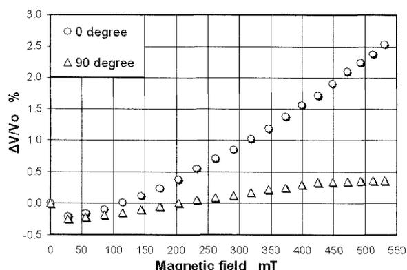
Fig. 5 Effect of angle on ultrasonic velocity propagation in MR fluid.
