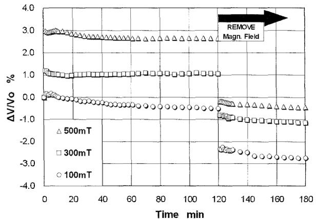
Fig. 4 The ultrasonic propagation velocity before and after removing the magnetic field in MR fluid.
