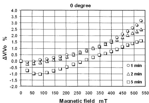
Fig. 6 The effect of interval time on the ultrasonic velocity propagation in MR fluid in  $0^\circ$  angle.
