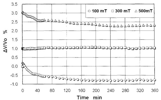
Fig. 3 Elapsed time dependence of ultrasonic propagation in MR fluid.
