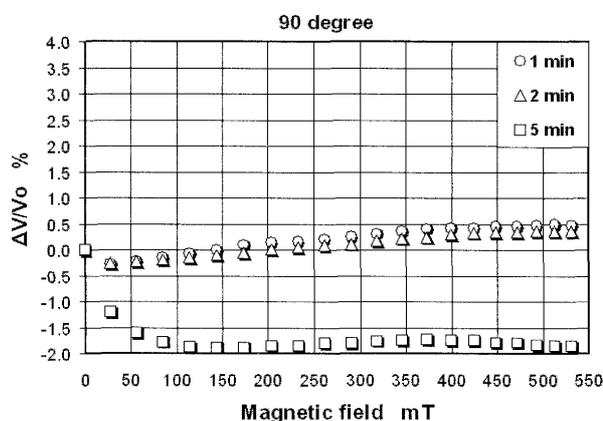
Fig. 7 The effect of interval time on the ultrasonic velocity propagation in MR fluid in  $90^\circ$  angles.
