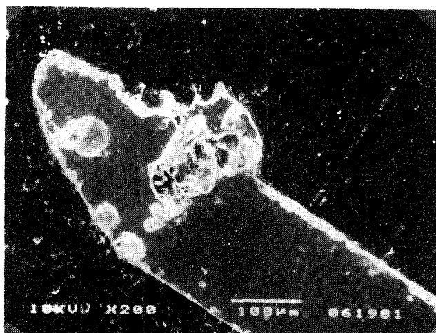
Fig. 4 SEM photomicrograph showing a cross section of a laser pit. Note that the diameter of the secondary frothy glass is larger than that of the pit.
