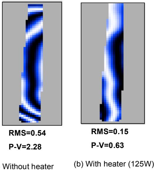
Fig.2. Cross sectional laser beam Interference patterns in the direction parallel to TIR surface as the result of zig-zag propagation through the slab medium. (a) 75 J pumping without heater. (b) With 125 W heating.
