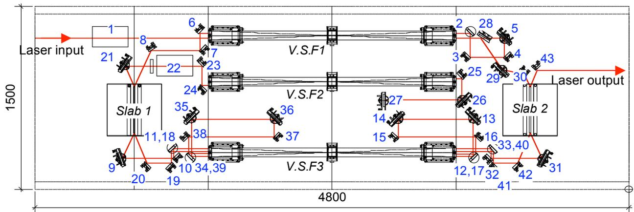
Fig. 3. A schematic diagram of the multi-pass optical amplifier layout. (1:Faraday isolator, 2-21:Mirror, 22:Faraday rotator, 23-27:Mirror, 28:Polarizer, 29-43:Mirror).
