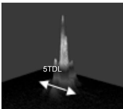
Fig. 5. FFP of laser output.
