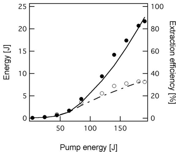
Fig. 4. Extraction energy from laser system of single amplifier configuration at 10 Hz. (Circle is experimental data with heating. Curve is computation data by used of modified Eggleston-Frantz model analysis.)
